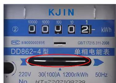
**Figure 12.** Metal rotary table of mechanical electricity meter.
