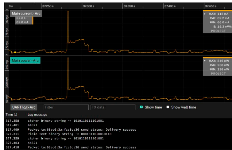
Figure 10. Power consumption measurement by Oti Arc.
