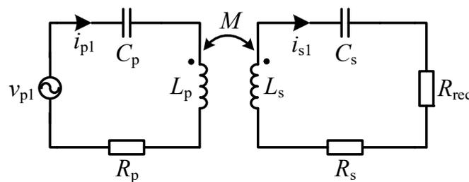
Figure 2. Equivalent system with the SS compensated circuit.
