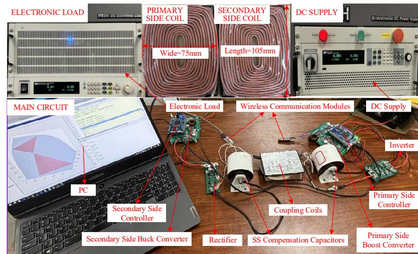
Figure 12. Physical image of the experimental platform.
