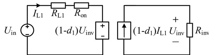
Figure 5. Simplified schematic diagram of the Boost converter.
