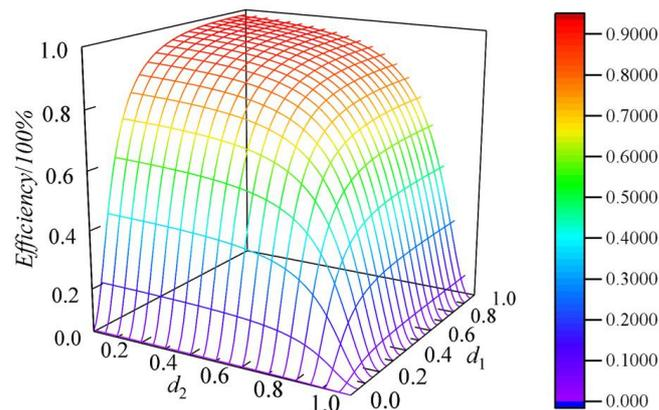
Figure 9. The relationship between the transmission efficiency of the multi-stage WPT system and the duty cycles  $d_1$  and  $d_2$ . Parameters are set as follows:  $f_s = 100$  kHz,  $M = 12.62$   $\mu$ H,  $R_{L1} = 11$  m $\Omega$ ,  $R_{on} = 10$  m $\Omega$ ,  $R_{L2} = 12$  m $\Omega$ ,  $R_p = 181.5$  m $\Omega$ , and  $R_s = 181.53$  m $\Omega$ .
