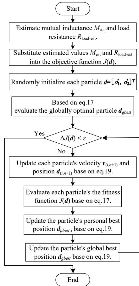
Figure 11. System optimization process based on PSO algorithm.
