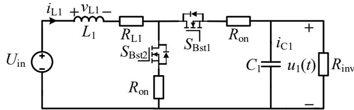
Figure 4. Schematic diagram of the Boost converter.
