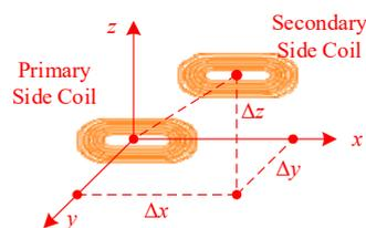
**Figure 14.** Diagram of coil spatial distance.
