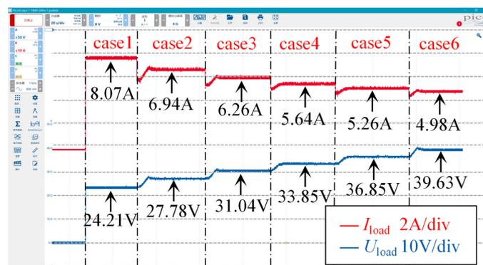
**Figure 15.** Results from the traditional resonance network impedance matching method.
