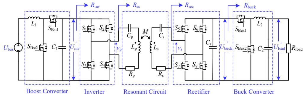
Figure 1. Circuit diagram of the multi-level DC-DC converter WPT system.
