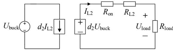
Figure 8. Simplified schematic diagram of the Buck converter.
