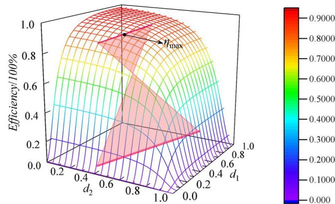
**Figure 10.** The relationships between the efficiency,  $d_1$  and  $d_2$ . ( $U_{in} = 28$  V,  $f_s = 100$  kHz,  $M = 12.62$   $\mu$ H,  $R_{L1} = 11$  m $\Omega$ ,  $R_{on} = 10$  m $\Omega$ ,  $R_{L2} = 12$  m $\Omega$ ,  $R_p = 181.5$  m $\Omega$ ,  $R_s = 181.53$  m $\Omega$ , and  $R_{load} = 8\Omega$ ).
