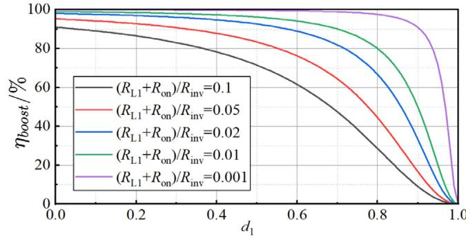
**Figure 6.** The relationship between  $\eta_{boost}$ ,  $d_1$ , and  $R_{inv}$ . ( $f_s = 100$  kHz,  $R_{L1} = 11$  m $\Omega$ , and  $R_{on} = 10$  m $\Omega$ ).
