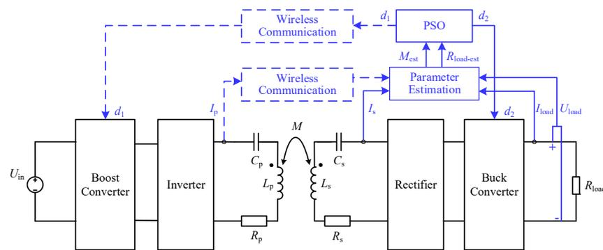
**Figure 13.** Principle diagram of multi-level joint efficiency optimization for WPT system using PSO algorithm.
