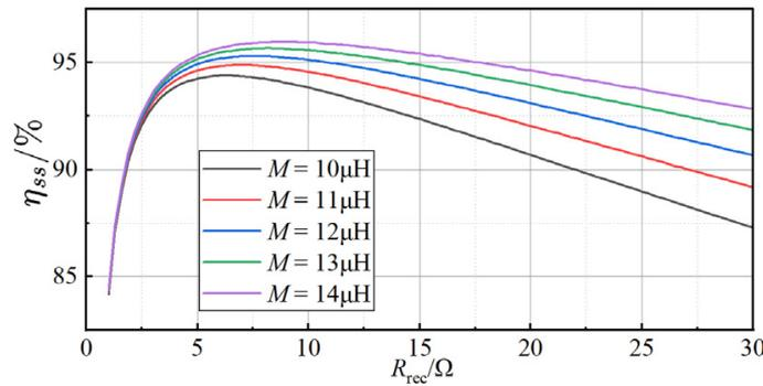
**Figure 3.** The relationship between the efficiency  $\eta_{ss}$ , load resistance  $R_{rec}$ , and mutual inductance  $M$  (where operating frequency  $f = 100$  kHz,  $R_p = 181.5$  mΩ,  $R_s = 181.53$  mΩ).
