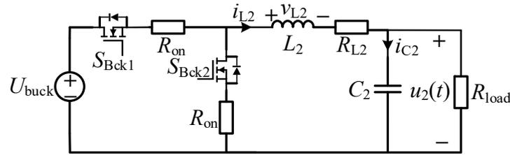
**Figure 7.** Schematic diagram of the Buck converter.
