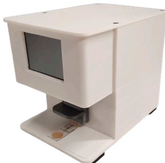
Figure 10. Design of the small-current measurement system casing. The evaluated OFET device is connected via the spring probes.
