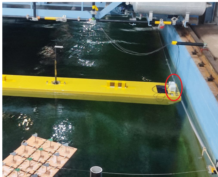
Figure 16. Sensor Node installed on the breakwater as tested during the wave basin tests.
