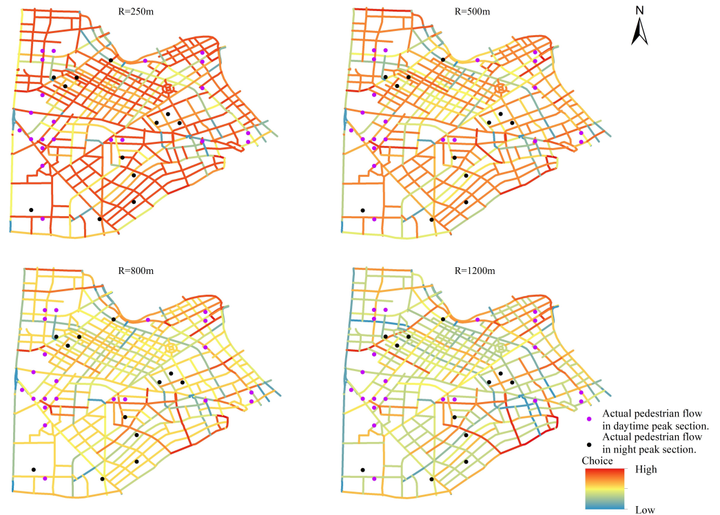
Figure 7. Comparison of connectivity degree and passenger flow density during morning and evening peak hours on weekdays.
