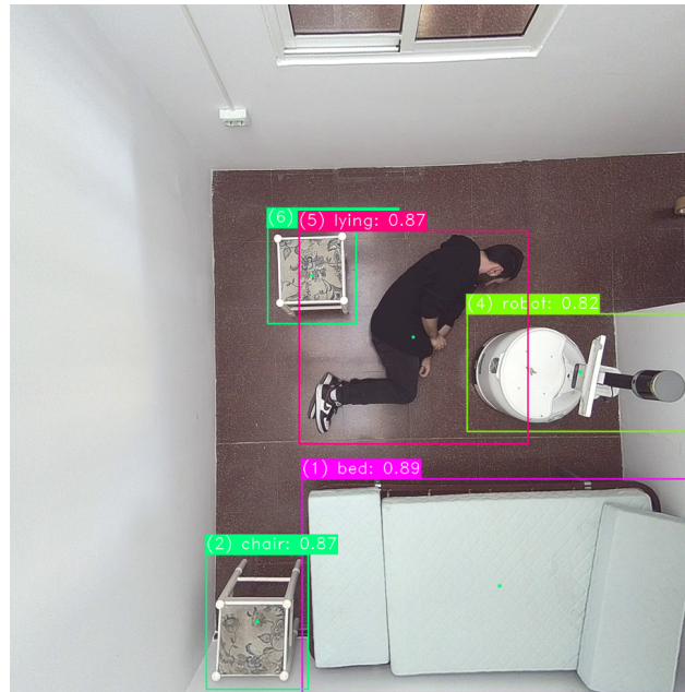
Figure 12. The detection of a person lying on the floor and objects (chairs and a bed) in the bedroom.
