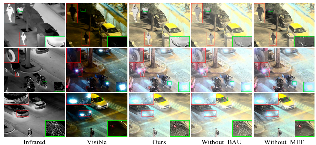
Figure 9. Visualized results of ablation on three typical infrared and visible image pairs. From top to bottom: infrared images, visible images, fused results of BMFusion, BMFusion without BAU, and BMFusion without MEF.
