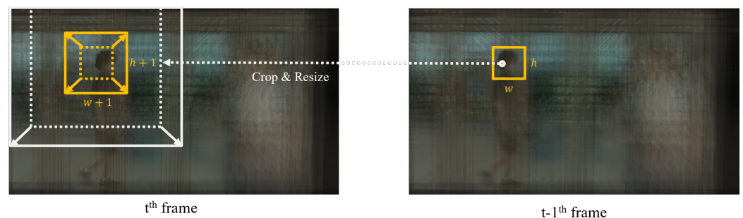
Figure 7. Dynamic change of spatial search region according to similarity score, which prevents an excessive change of search region for the next prediction.
