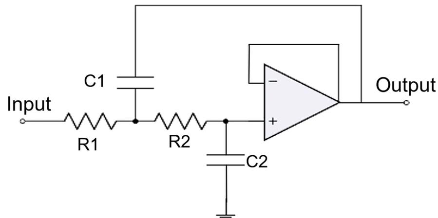
**Figure 11.** Circuit diagram for the low-pass SK filter.
