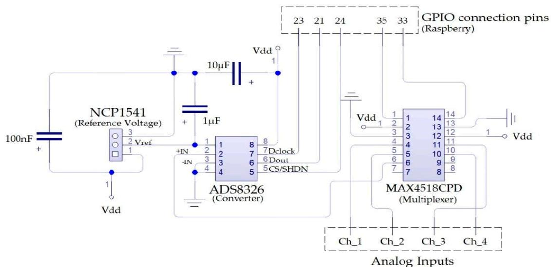
**Figure 1.** Schematic of the DAQ board presented in ref. [3].
