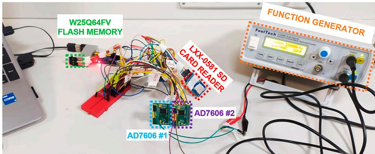
Figure 16. Setup employed for the DAQ prototype.
