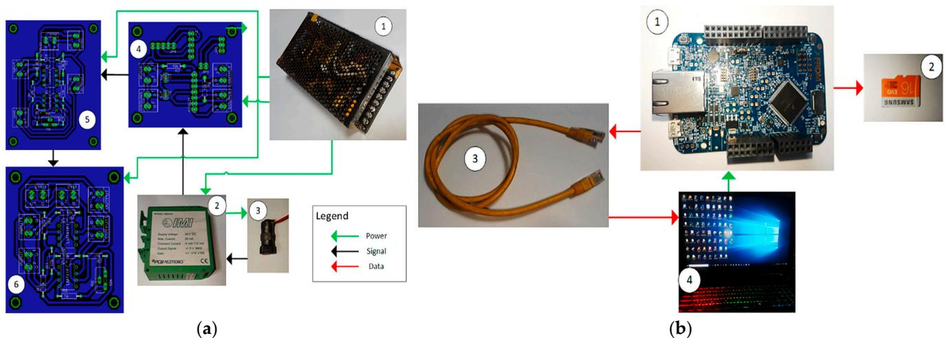
**Figure 2.** Analog section (a) of the system proposed in ref. [14] with highlighted the power supply (1), signal conditioner (2), accelerometer (3), active antialiasing filter (4), diode clipper circuit (5), and the Direct-Current voltage bias circuit (6); the digital section (b) of the designed solution with highlighted the development board (1), MicroSD card (2), Ethernet cable (3), and the laptop (4).
