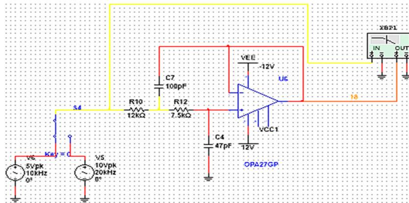
Figure 12. Multisim schematic for the implemented SK antialiasing filter.
