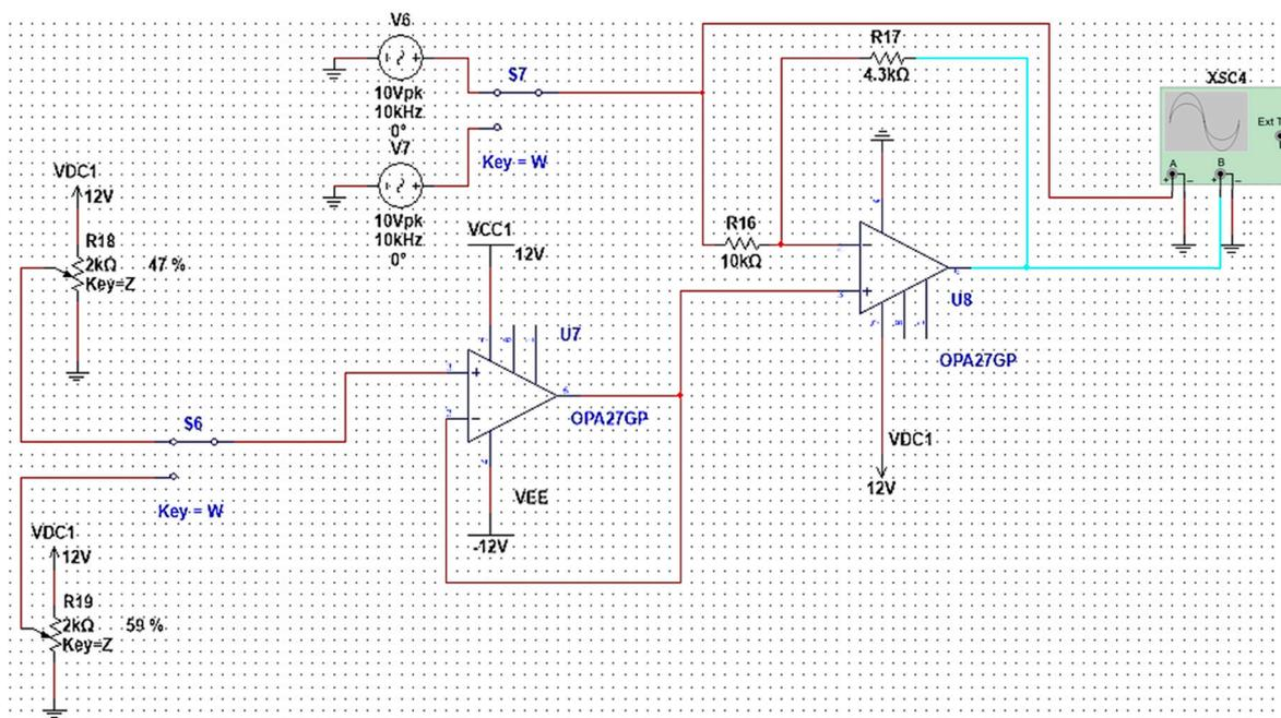
Figure 9. Multisim setup for the implemented level shifter. As stated before, two cases are considered for the DC component of the input signal, i.e., when  $V_{IN}$  is equal to 7.1 V and 12 V.
