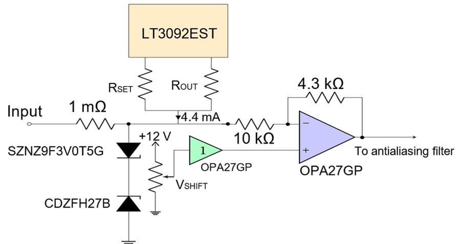
Figure 7. Functional block diagram of the signal conditioning chain for “MODE 2”.
