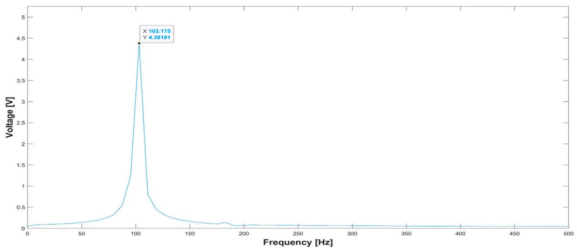
Figure 28. SSB FFT of the low-frequency vibrational signals acquired by the DAQ board prototype (in the makers, X represents the frequency and Y represents the harmonic component amplitude).
