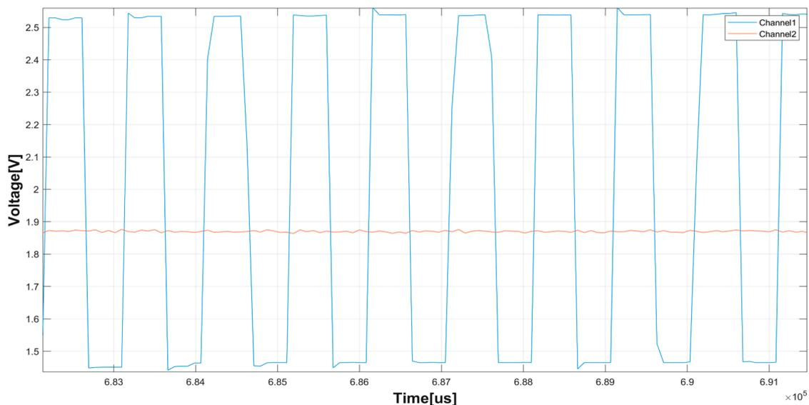
**Figure 21.** Waveforms acquired by the developed DAQ system prototype on channel 1 (500 Hz square wave, blue trace) and channel 2 (1.87 V DC voltage, orange trace).
