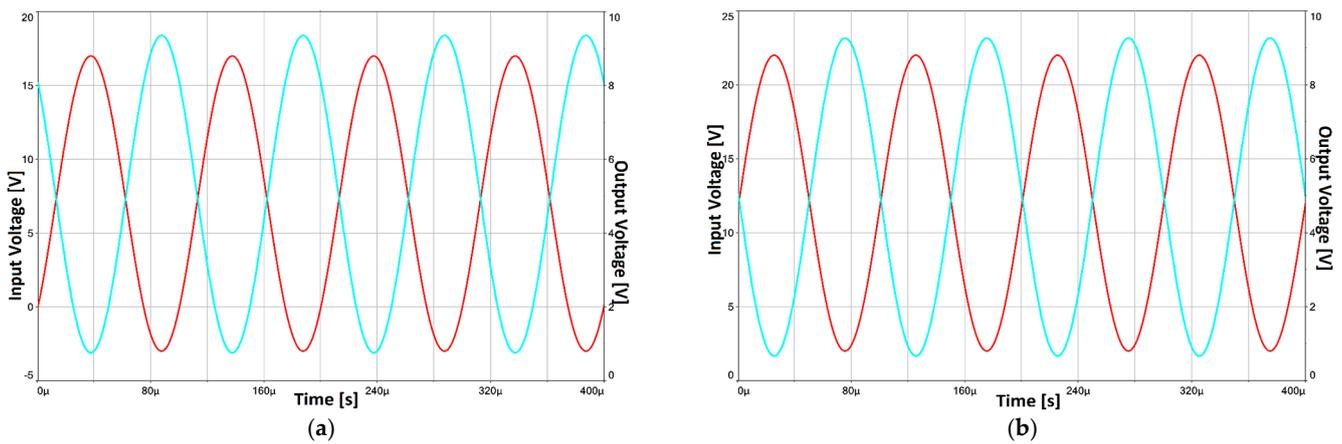
**Figure 10.** Results of the simulations for the proposed level shifter on Multisim (the red trace is the input signal, the light blue one is the output signal). (a)  $V_{IN}$  equal to 7.1 V and  $V_{SHIFT}$  equal to 5.6 V; (b)  $V_{IN}$  equal to 12 V and  $V_{SHIFT}$  equal to 7.1 V.
