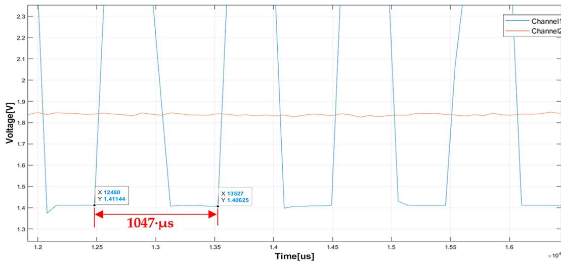
**Figure 22.** Detailed view of the waveforms acquired by the developed DAQ system prototype on channels 1 (1 kHz square wave, blue trace) and 2 (1.87 V DC voltage, orange trace), with the period of the square wave emphasized (1.047 ms).
