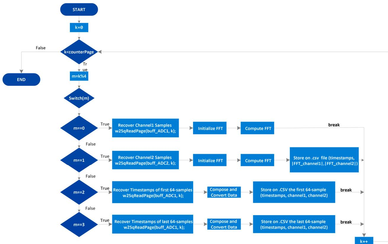
Figure 20. Flowchart related to the data recovery from flash memory, FFT calculation, and data storage into CSV files on the SD card.
