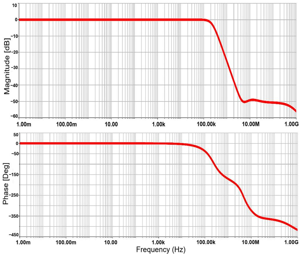
Figure 13. Bode plots for magnitude and phase responses of the simulated antialiasing filter. It is worth observing that these Bode plots are valid for both filter inputs, and the filter introduces two poles at approximately  $f_{3dB}$ , resulting in a  $-40$  dB/decade attenuation.
