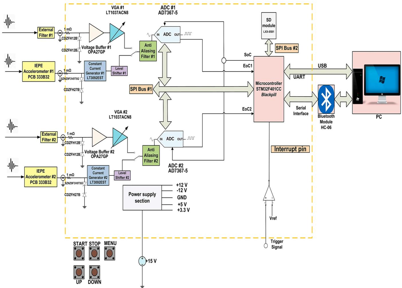
Figure 3. Block diagram for the proposed acquisition board.
