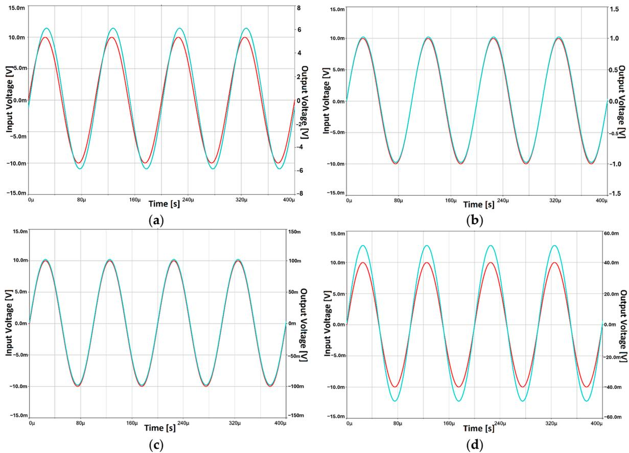
**Figure 6.** Simulations of VGA carried out with Multisim. The red trace is the input signal, and the blue one is the output signal for different set gains: (a) 600 V/V, (b) 100 V/V, (c) 10 V/V, and (d) 5 V/V.
