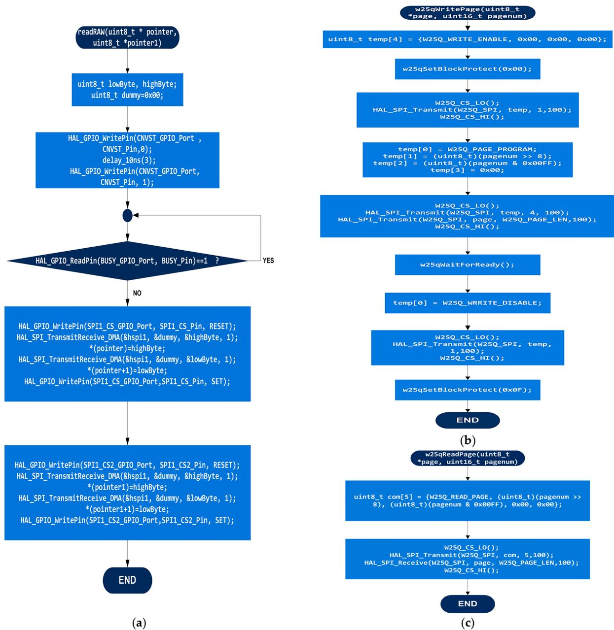
Figure 19. Flowchart of the following methods: (a) *readRAW()*, (b) *w25qWritePage()*, and (c) *w25qReadPage()*.
