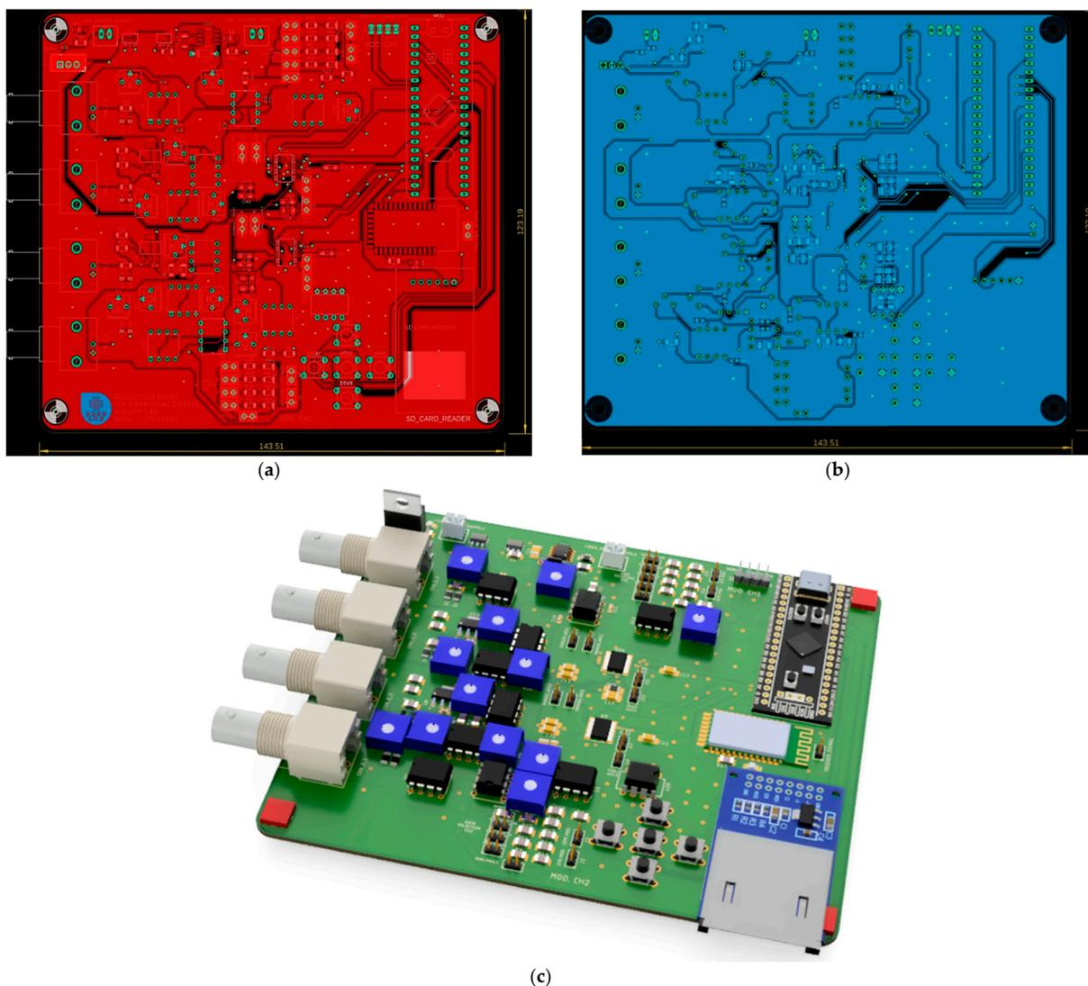
Figure 14. (a) Top, (b) bottom, and (c) 3D views of the designed acquisition board.
