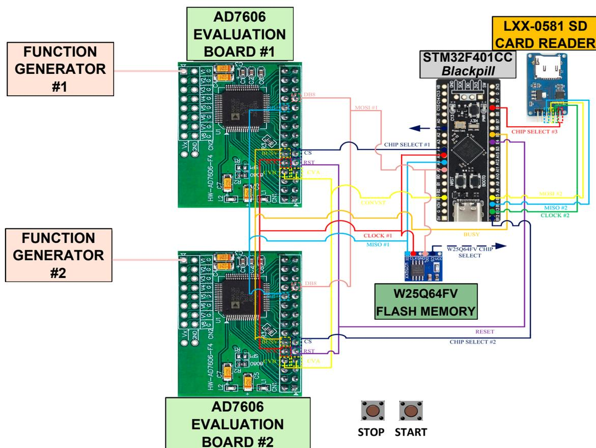
Figure 15. DAQ prototype's schematic.
