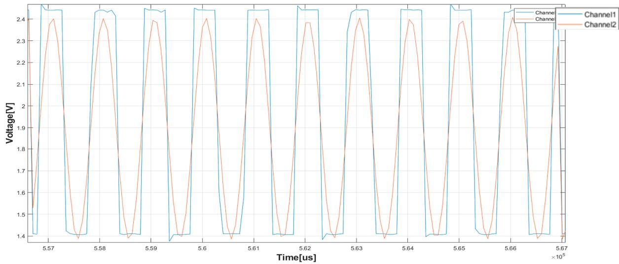
**Figure 23.** The developed DAQ system prototype acquired waveforms on channel 1 (1 kHz square wave, blue trace) and channel 2 (1 kHz sine wave, orange trace).
