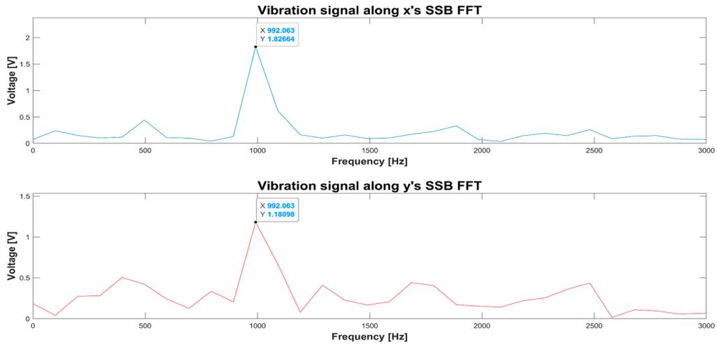
Figure 26. SSB FFT of the vibrational signals acquired by the DAQ board: *x*-axis (blue trace) and *y*-axis (red trace) signals (in the makers, X represents the frequency and Y represents the harmonic component amplitude).
