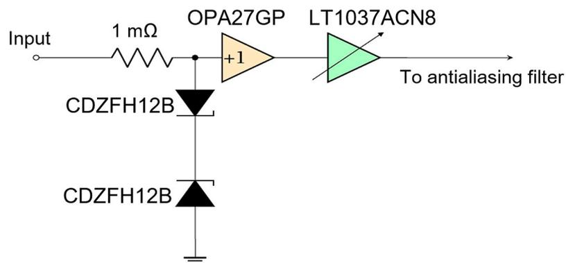
Figure 4. Functional block diagram for the signal conditioning chain for “MODE 1”.
