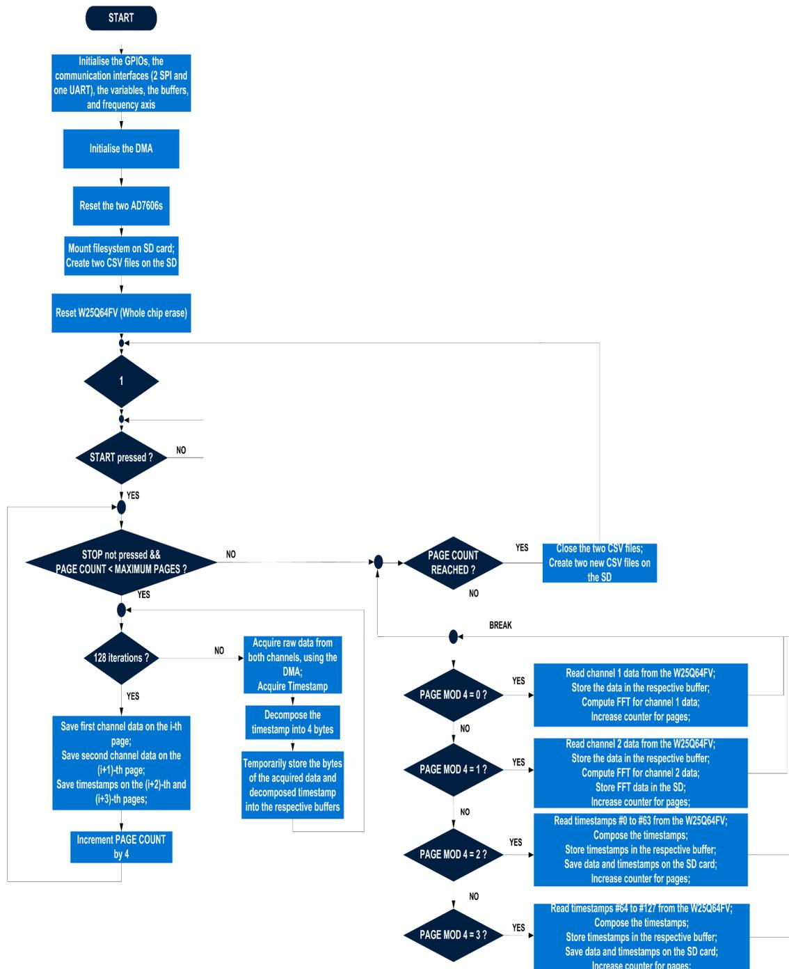
Figure 17. High-level flowchart for the firmware developed for the prototype board based on the AD7606.
