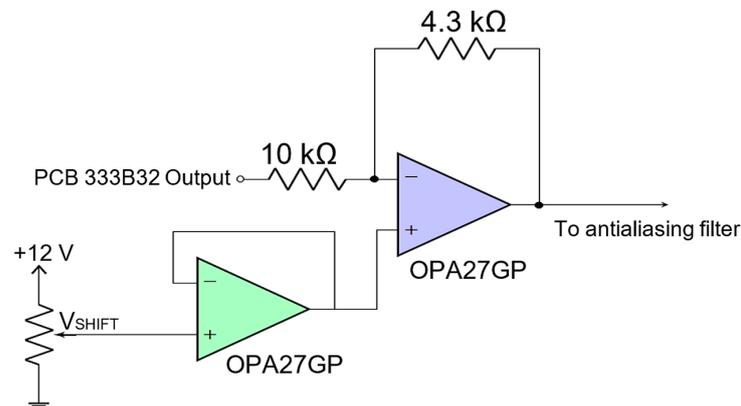
Figure 8. Circuit diagram of the designed level shifter.
