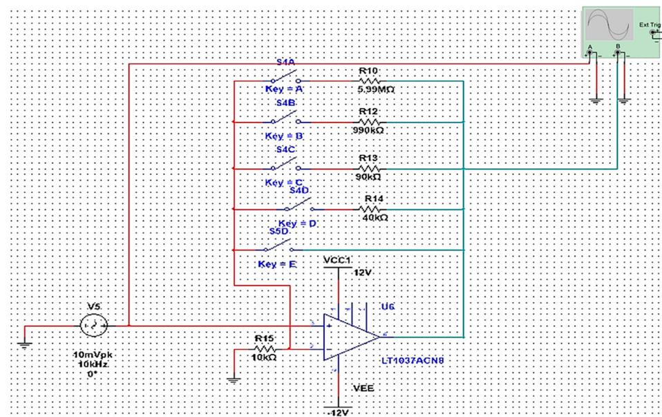
Figure 5. Multisim setup for the implemented VGA. The VGA is designed assuming a sinusoidal input signal with a 10 mVpk amplitude and a 10 kHz frequency as the input.
