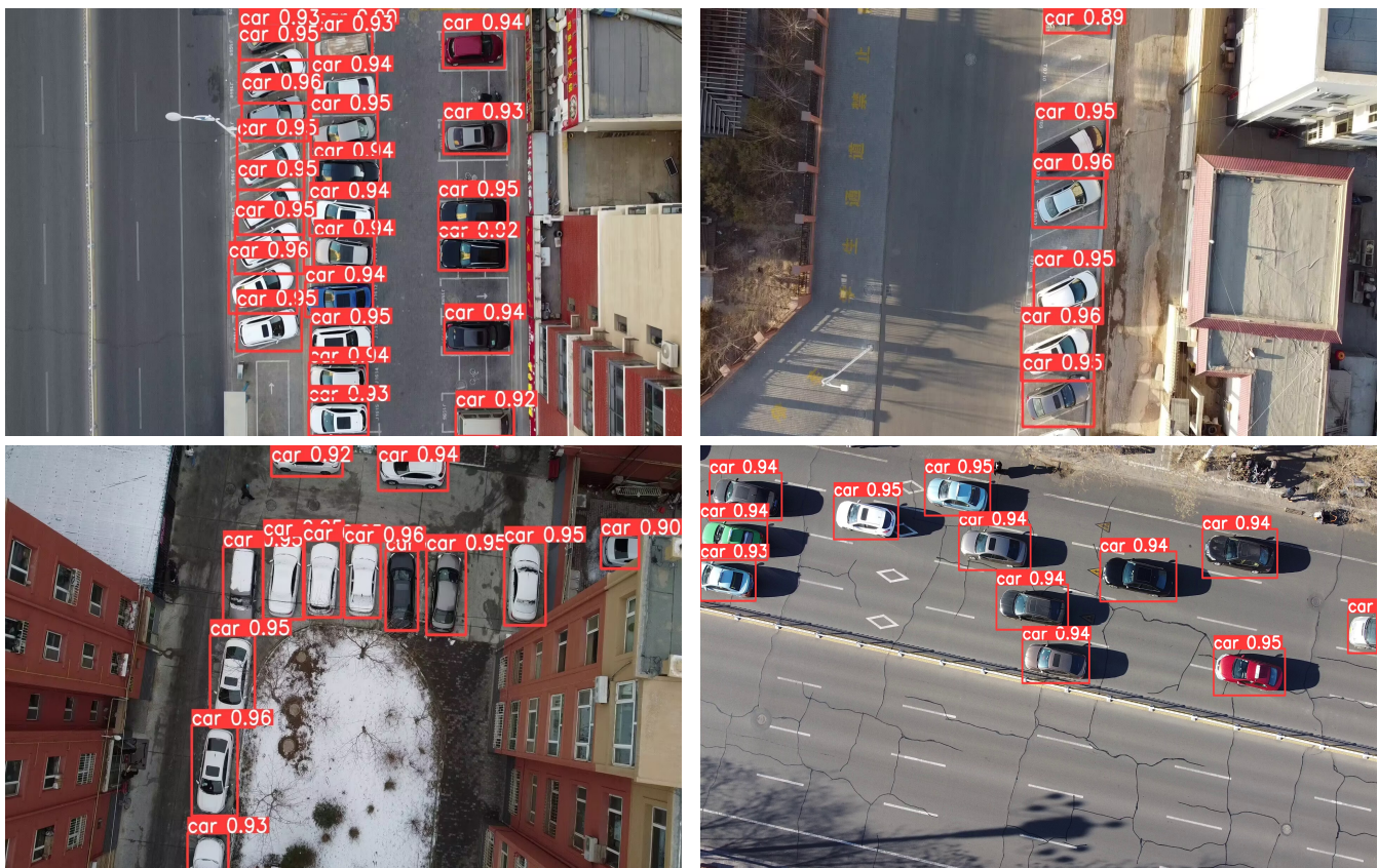
Figure 12. Visual demonstrations of precise vehicle detection across diverse backgrounds in the UAV-ROD dataset.
