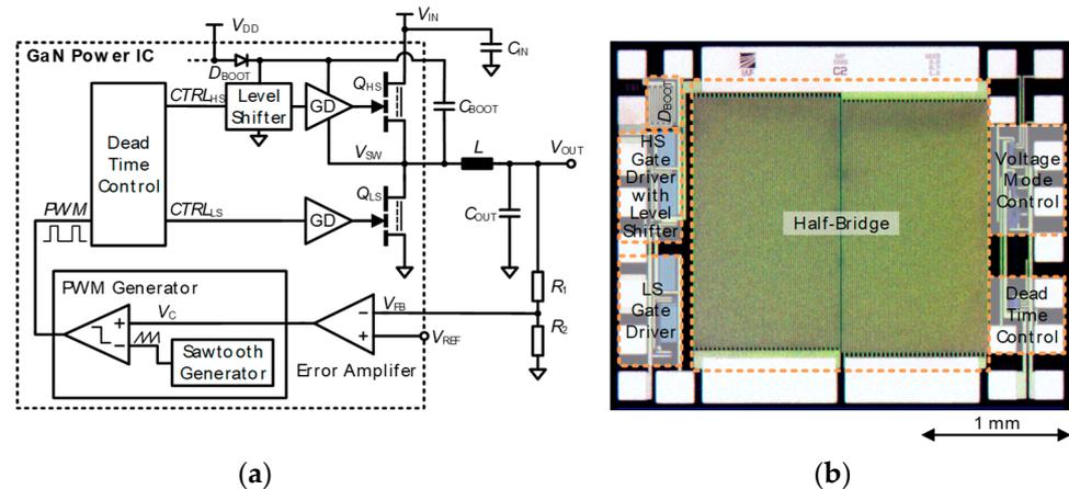
**Figure 1.** GaN power stage for 48 V DC-DC converters consisting of a half-bridge with driver, level shifter, dead time control and voltage mode control. (a) Schematic and (b) chip photo.
