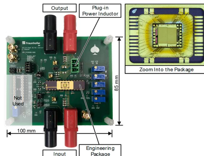
**Figure 2.** Experimental setup of the GaN IC ( $3 \times 2.5 \text{ mm}^2$ ) in the DIL engineering package, which is plugged into an adapter on a DC–DC converter board. In addition, an inset is shown of the zoom into the package.
