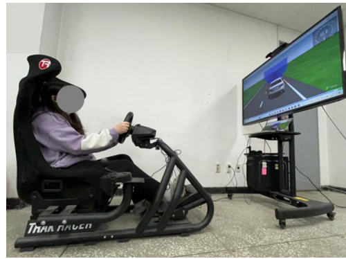
Figure 12. Driving characteristics data acquisition experiment environment.
