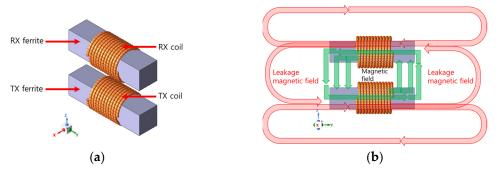
Figure 2. Structure of dipole-type WPT coils: (a) bird's-eye view and (b) the shape of the magnetic field.
