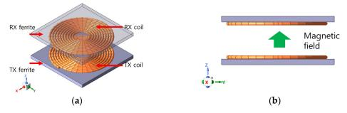
Figure 1. Structure of typical planar WPT coils: (a) bird's-eye view and (b) the shape of the magnetic field.
