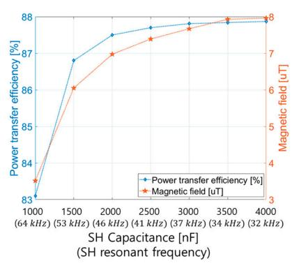
**Figure A1.** Changes in power transfer efficiency and leakage magnetic field according to changes in SH side capacitance.
