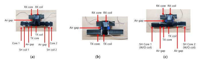
**Figure 12.** Dipole coil structures fabricated to validate the effectiveness of the reactive shield proposed through experiments: (**a**) proposed structure, (**b**) comparison Case 1—case with long TX ferrite, and (**c**) comparison Case 2—case in which only SH ferrite is added.
