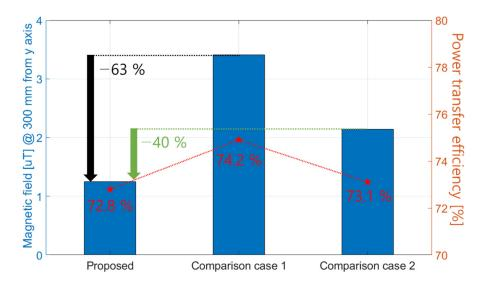
**Figure 17.** Comparison of the magnetic field and power transfer efficiency of the proposed model and comparison groups.
