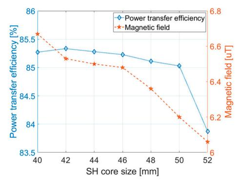
**Figure A5.** Changes in power transfer efficiency and leakage magnetic field according to changes in SH core size.
