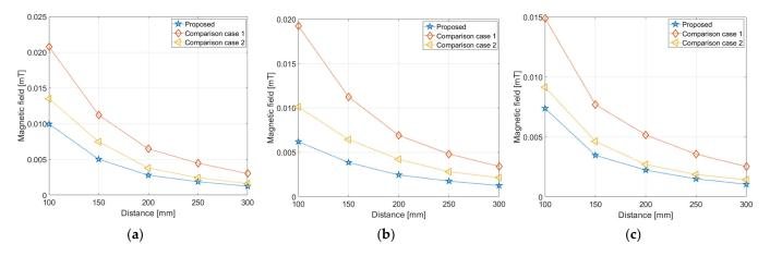
**Figure 16.** Magnetic field measurement results depending on the distance from the WPT coil system: (a) *x*-axis, (b) *y*-axis, and (c) *z*-axis.
