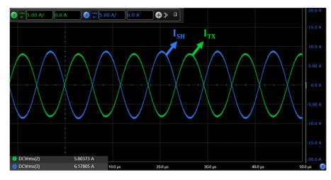
Figure 14. Measurement results of TX and SH coil currents in the proposed model.
