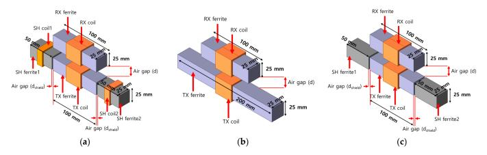
**Figure 8.** Simulation illustration of the proposed reactive shield structure and comparison groups: (a) proposed structure; (b) comparison Case 1—case with long TX ferrite; (c) comparison Case 2—case in which only SH ferrite is added.
