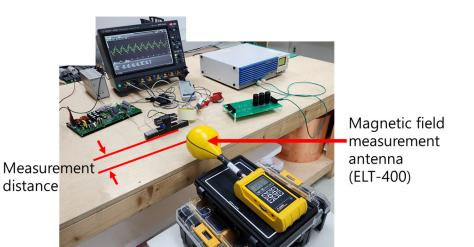
Figure 15. Measurement of the magnetic field from the WPT coil.
