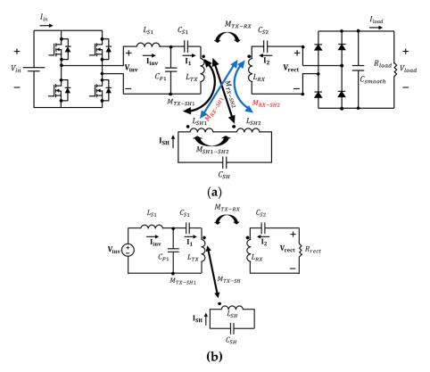
**Figure 4.** WPT equivalent circuit with proposed reactive shield structure: (**a**) actual circuit diagram and (**b**) simplified equivalent circuit considering only AC components.
