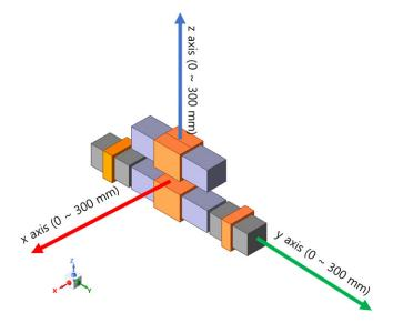
Figure 9. Magnetic field measurement for leakage magnetic field simulation.
