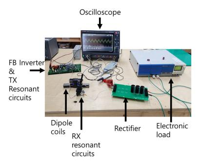
Figure 13. Setup for wireless power transfer experiments.
