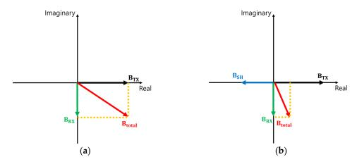
**Figure 6.** Vector sum of magnetic fields in the WPT coil: (**a**) vector sum when SH coil is not applied and (**b**) vector sum when SH coil is applied.
