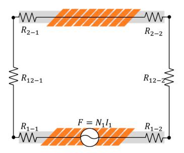
Figure A3. A typical dipole coil structure modeled as a magnetic circuit.
