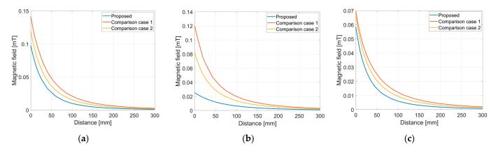
**Figure 10.** Magnetic field simulation results for each axis of the proposed reactive shield model and comparison groups: (**a**) *x*-axis, (**b**) *y*-axis, and (**c**) *z*-axis.
