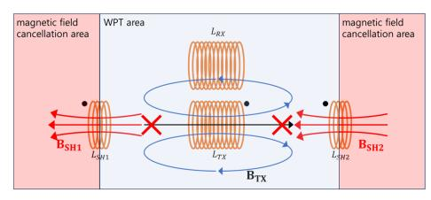
**Figure 7.** Magnetic field configuration according to the area in the reactive shield structure for the proposed dipole structure.
