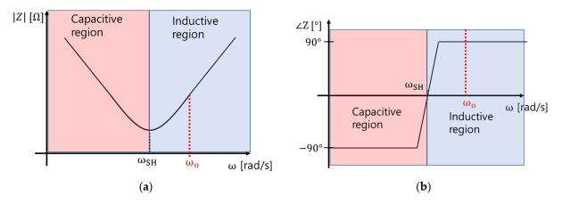
**Figure 5.** Impedance comprising the SH coil ( $L_{SH}$ ) and resonant circuit ( $C_{SH}$ ): (**a**) impedance magnitude and (**b**) impedance phase.
