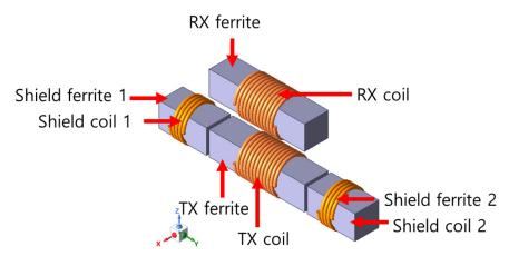
Figure 3. Dipole-type WPT coil with the proposed reactive shield.
