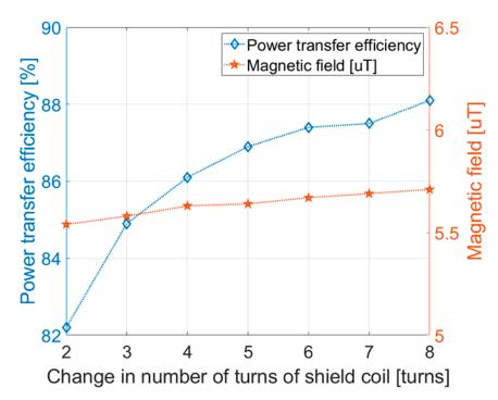
**Figure A2.** Changes in power transfer efficiency and leakage magnetic field according to changes in SH coil turns.
