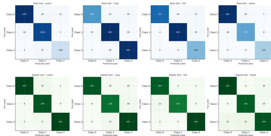
Figure 7. Confusion matrix results for Random Forest (RF): real soil (top row) vs. digital twin (bottom row).
