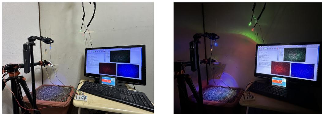
**Figure 2.** Experimental setup for real soil: **(Left)** Indoor setup for soil moisture analysis with LED lighting and real-time data display. **(Right)** Low-light indoor setup capturing soil properties with LED lighting for digital twin modeling.
