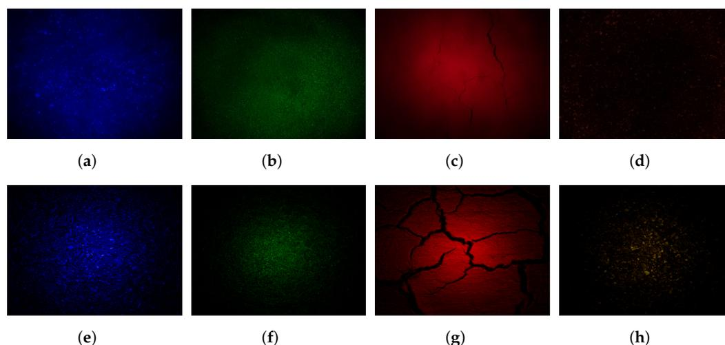
**Figure 4.** Comparison of real soil images (top row) and digital twin images (bottom row) across different color channels: (a,e) blue; (b,f) green; (c,g) red; (d,h) yellow.
