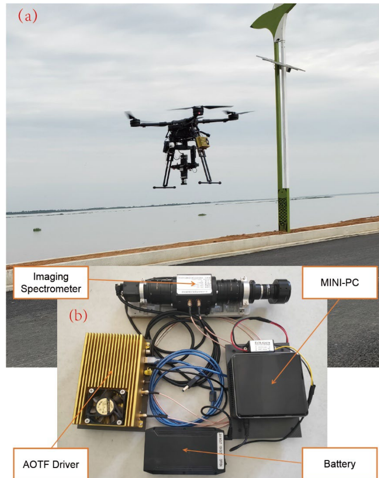
Figure 1. Composition of the unmanned aerial vehicle (UAV)-mounted hyperspectral imaging system based on the airborne acousto-optic tunable filter (AOTF) spectrometer. (a) Components of the imaging system included the AOTF spectrometer, AOTF driver, MINI-PC, and battery. (b) AOTF spectrometer airborne imaging system featuring a zoom lens.
