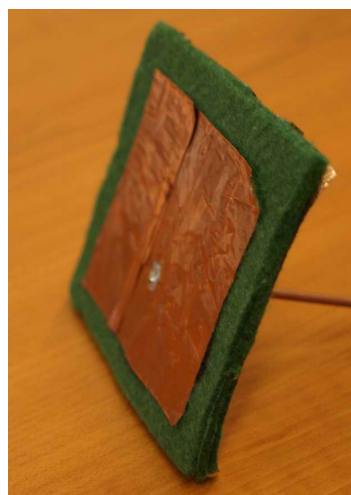
Figure 3. Textile patch antenna (substrate: felt, conducting sections: copper tape) with partially detached copper tape due to environmental conditions.
