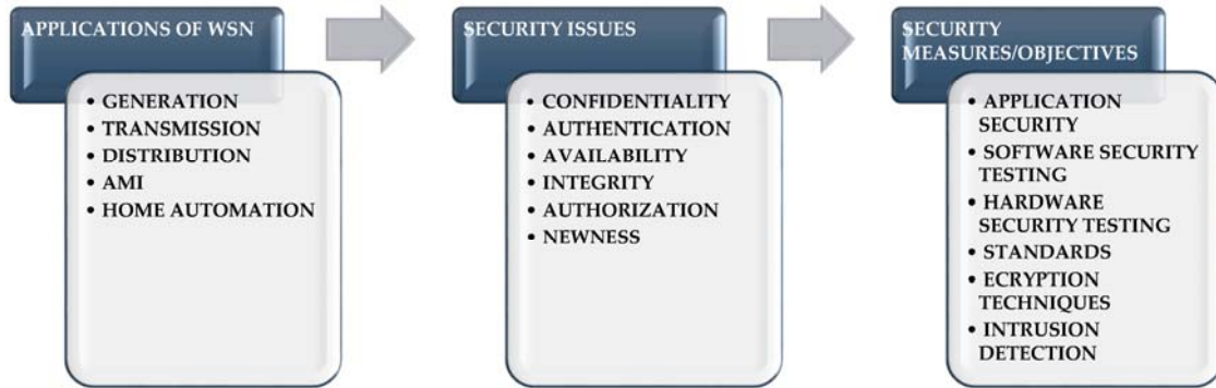
Figure 4. An overview of applications, security issues and security measures for WSN based smart grid architecture.
