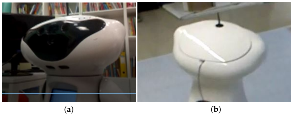
Figure 2. Head of the MONarCH robot (with the RFID reader hidden inside). (a) lateral view without head cover; (b) top view with the head cover in place.
