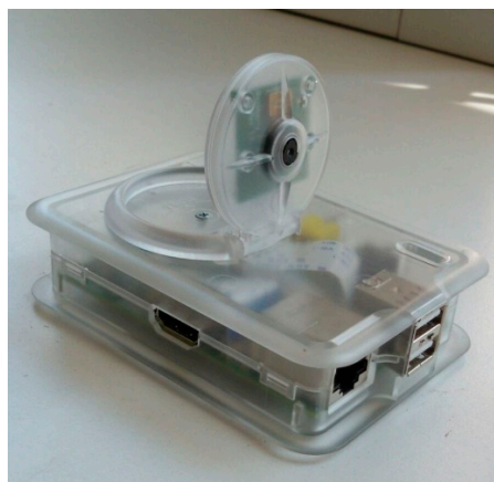
Figure 2. Image acquisition subsystem (Raspberry Pi 2 Model B and Pi camera), standalone configuration.
