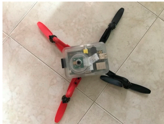
Figure 3. Image acquisition subsystem mounted on RC EYE One Xtreme.
