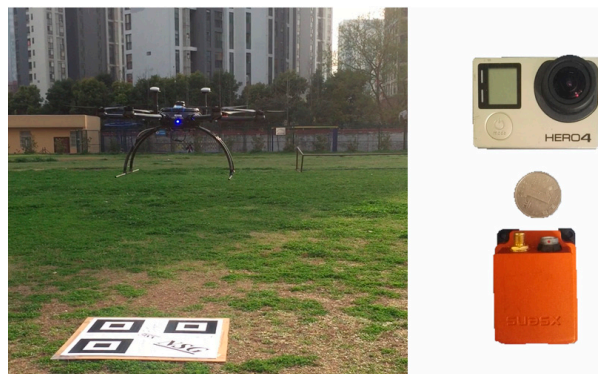
Figure 5. Left: Landing object RQRLP and the employed six-rotors aircraft system. Right: Onboard camera and the Inertial Measurement Unit (IMU) module.
