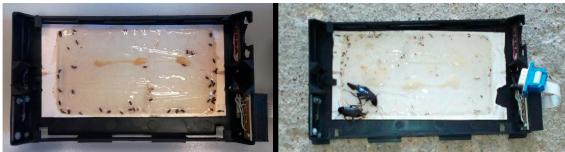
Figure 5. Evaluation of reported results. Sticky surface inside the trap after 2 days of placement in (Left) a cereal grain storage facility with serious insect infestations, (Right) in an old food warehouse with an increased presence of cockroaches.
