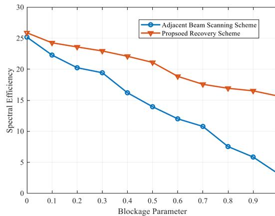
Figure 4. Spectral efficiency for various blockage parameters.
