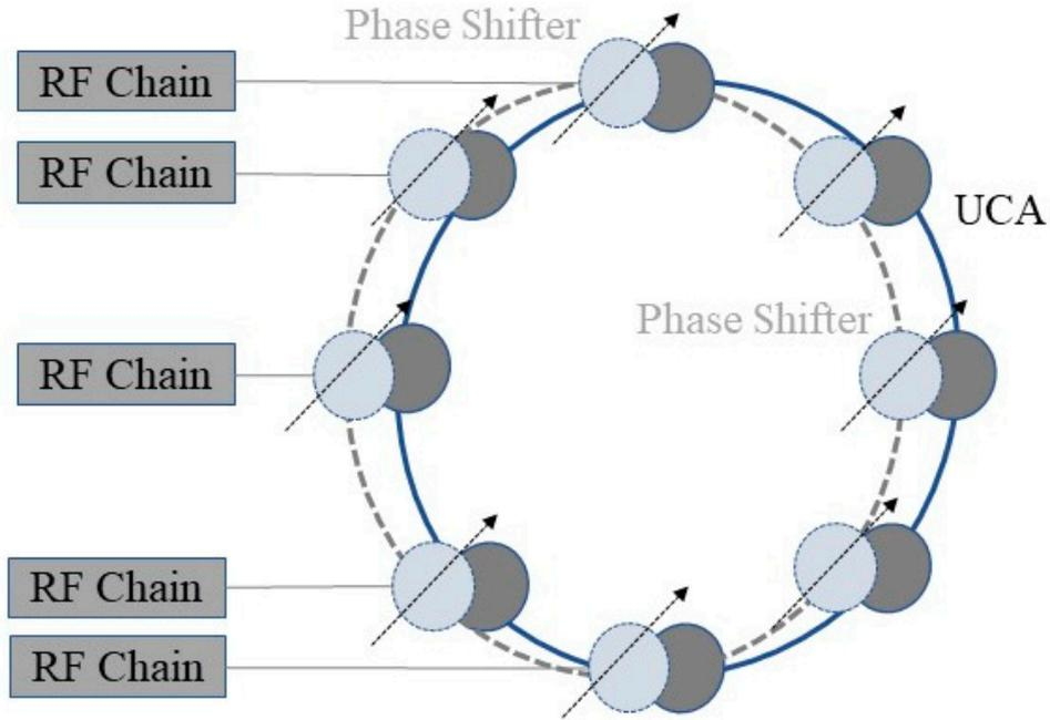
Figure 2. Digital beamformer at the BS.
