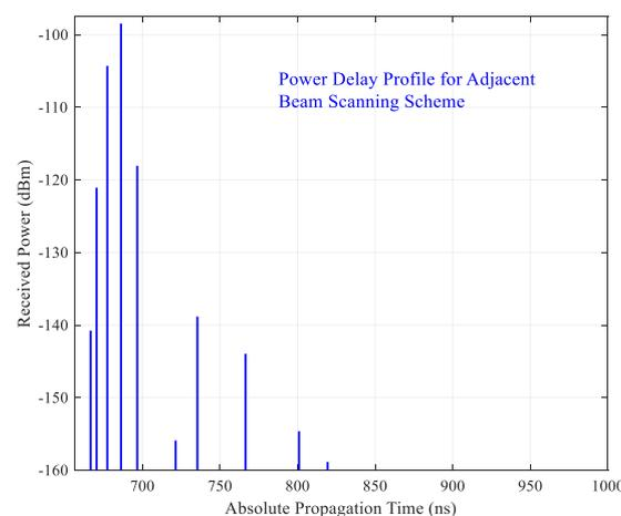
Figure 5. Power delay profile for conventional schemes (adjacent beam and aggregation).
