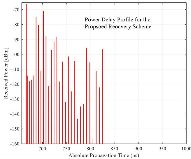
Figure 6. Power delay profile for proposed multi-backup scheme.
