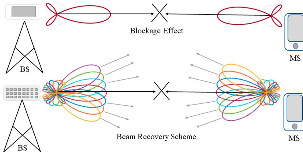
Figure 3. Proposed multi-backup beam recovery scheme.
