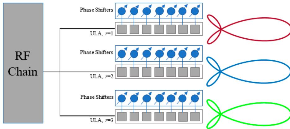
Figure 1. Proposed parallel analog beamformer.
