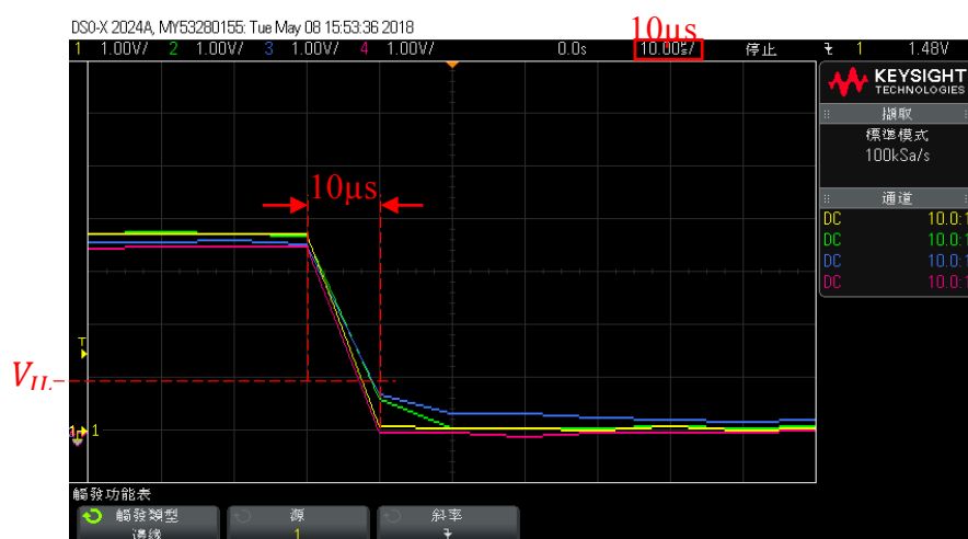
Figure 21. The time synchronization experiment assisted by PPS (pulse-per-second) of GPS (global positioning system).
