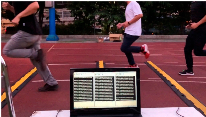
Figure 19. Four runners with a BLE Tag on their respective insteps ran through the three sets of MAT one by one.
