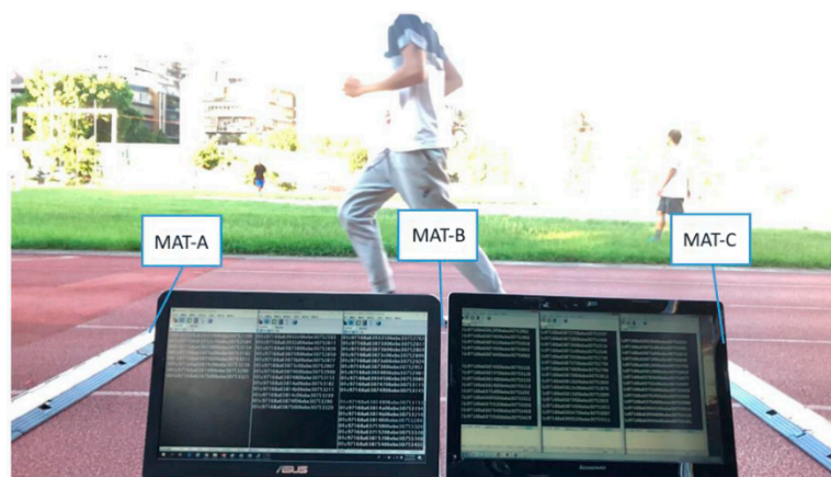
Figure 17. The dynamic experiment of three sets of MAT when a BLE Tag is on the runner’s chest.
