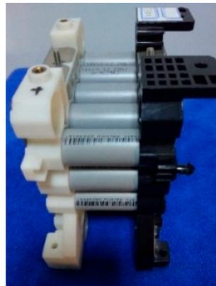
Figure 5. Battery module with 13 cells connected in parallel.
