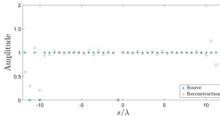
**Figure 14.** Reconstruction of a 41-element array with two faulty elements. The number of array elements is smaller than the one estimated by (17) as the source NDF (45).
