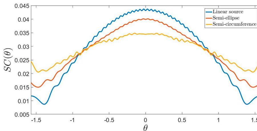
**Figure 15.** Spectral content functions  $SC(\theta)$  for a linear source ( $a'_x = 9.75 \lambda$ ), a semi-ellipse ( $a'_x = 8.75 \lambda$  and  $a'_z = 5 \lambda$ ), and a semi-circumference ( $a''_x = a''_z = 7.4 \lambda$ ) with the same number of significant eigenvalues ( $N_T = 40$ ).
