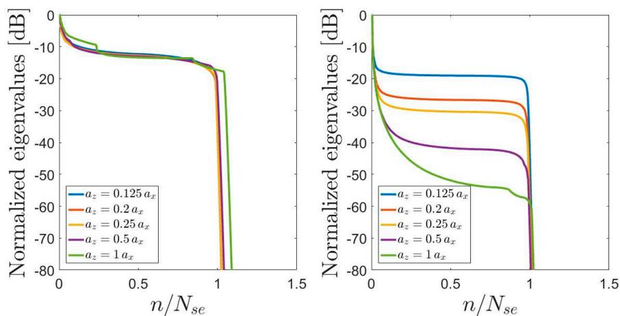
**Figure 10.** Normalized eigenvalue behaviors (reported in descending order) of  $\mathcal{L}_\theta$  (left panel) and  $\mathcal{L}_u$  (right panel) operators for a semi-elliptic source when  $a_x = 100\lambda$ . Each line refers to a different aspect ratio  $a_x/a_z$ .
