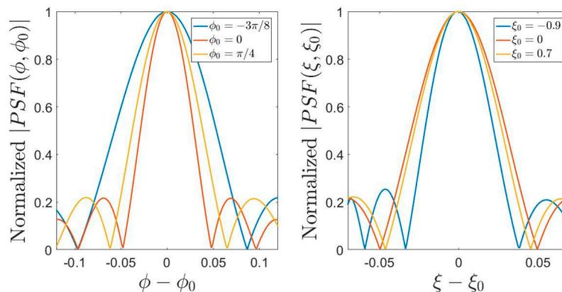
**Figure 11.** Normalized and overlapped PSFs of  $\mathcal{L}_\theta$  (left panel) and  $\mathcal{L}_u$  (right panel) operators of a semi-elliptic source, with  $a_x = 10\lambda$  and  $a_z = 5\lambda$ , for  $\phi_0 = -3\pi/8, 0, \pi/4$  and for the corresponding values  $\xi_0 = -0.9, 0, 0.7$ .
