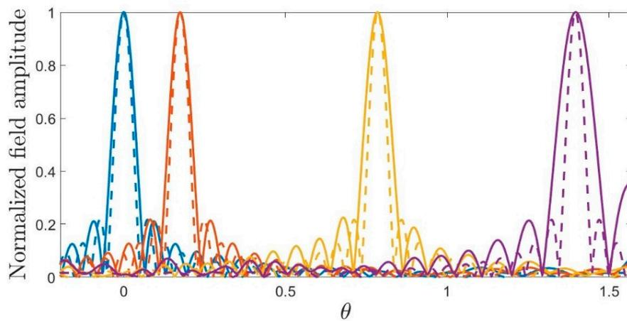
**Figure 18.** Normalized field amplitude of the desired field  $E(\theta)$  (dashed curves) and the projected field  $\tilde{E}(\theta)$  (solid curves) for the semi-circumference source, varying the main beam angle  $\theta_0 = 0, 0.17, 0.78, 1.4$ . The panels only zoom into a portion of the observation domain.
