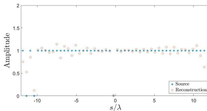
**Figure 13.** Reconstruction of a 50-element array with two faulty elements. The number of array elements is larger than the one estimated by (17) as the source NDF (45).
