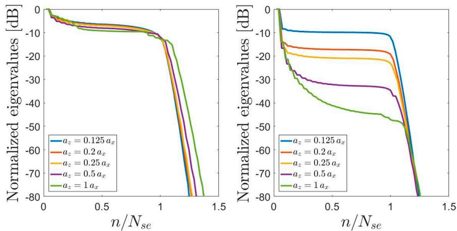
**Figure 9.** Normalized eigenvalue behaviors (reported in descending order) of  $\mathcal{L}_\theta$  (left panel) and  $\mathcal{L}_u$  (right panel) operators for a semi-elliptic source when  $a_x = 10\lambda$ . Each line refers to a different aspect ratio  $a_x/a_z$ .
