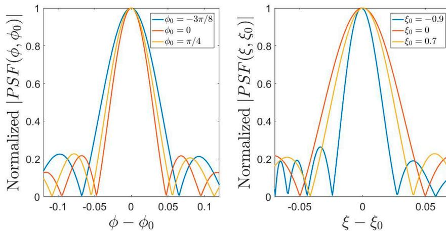
**Figure 6.** Normalized and overlapped PSFs of  $\mathcal{L}_\theta$  (left panel) and  $\mathcal{L}_u$  (right panel) operators of a semi-circumference source with  $a_x = 10\lambda$  for  $\phi_0 = -3\pi/8, 0, \pi/4$  and for the corresponding values  $\xi_0 = -0.9, 0, 0.7$ .
