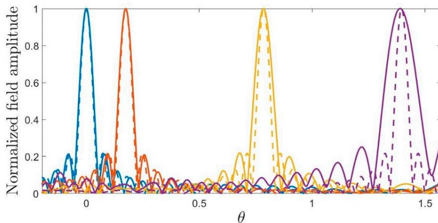
**Figure 17.** Normalized field amplitude of the desired field  $E(\theta)$  (dashed curves) and the projected field  $\tilde{E}(\theta)$  (solid curves) for the semi-elliptic source, varying the main beam angle  $\theta_0 = 0, 0.17, 0.78, 1.4$ . The panels only zoom into a portion of the observation domain.
