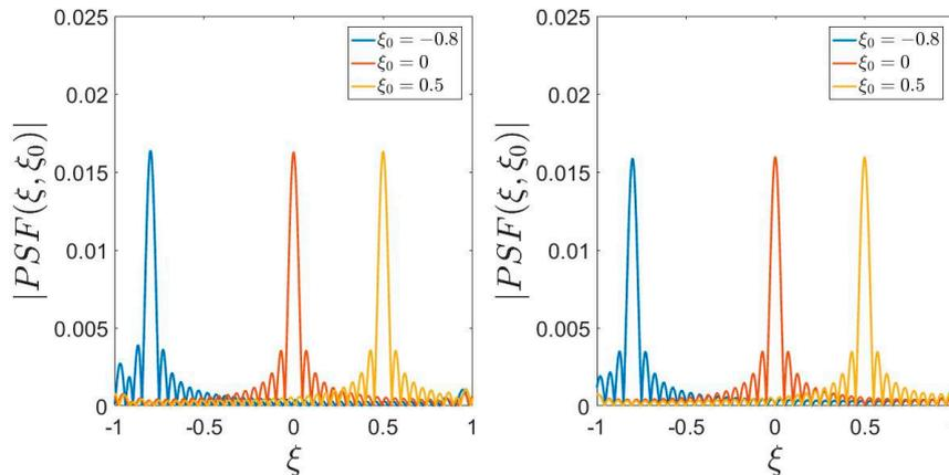
**Figure 2.** The point spread functions (PSFs) of the operators  $\hat{\mathcal{L}}_\theta$  (left panel) and  $\mathcal{L}_u$  (right panel) of a linear source with  $a_x = 10 \lambda$ , for  $\xi_0 = -0.8, 0, 0.5$ .
