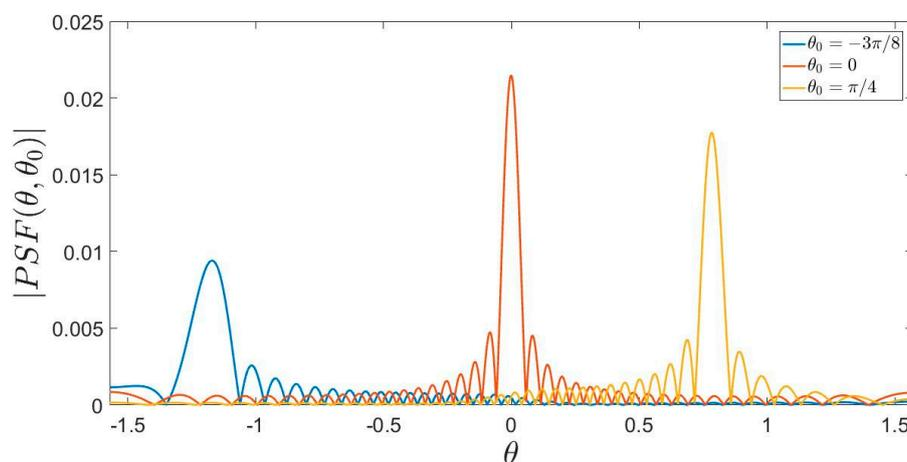
**Figure 3.** The PSF in the observation domain of the operator  $\hat{\mathcal{L}}_\theta$  of a linear source with  $a_x = 10\lambda$ , for  $\theta_0 = -3\pi/8, 0, \pi/4$ .
