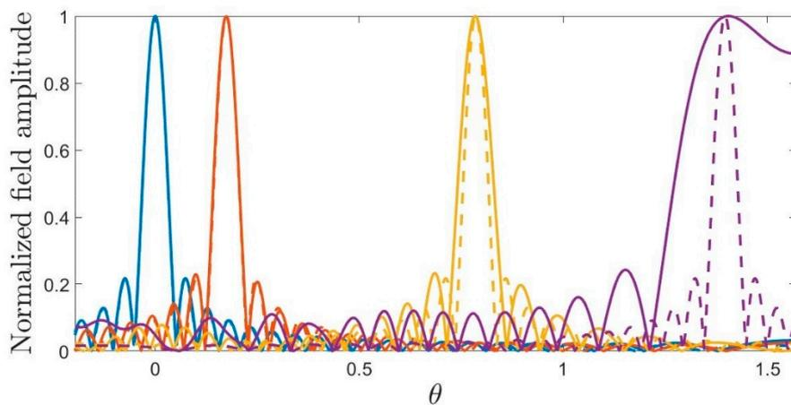
**Figure 16.** Normalized field amplitude of the desired field  $E(\theta)$  (dashed curves) and the projected field  $\tilde{E}(\theta)$  (solid curves) for the linear source, varying the main beam angle  $\theta_0 = 0, 0.17, 0.78, 1.4$ . The panels only zoom into a portion of the observation domain.
