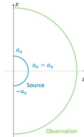
Figure 4. Semi-circumference source geometry.
