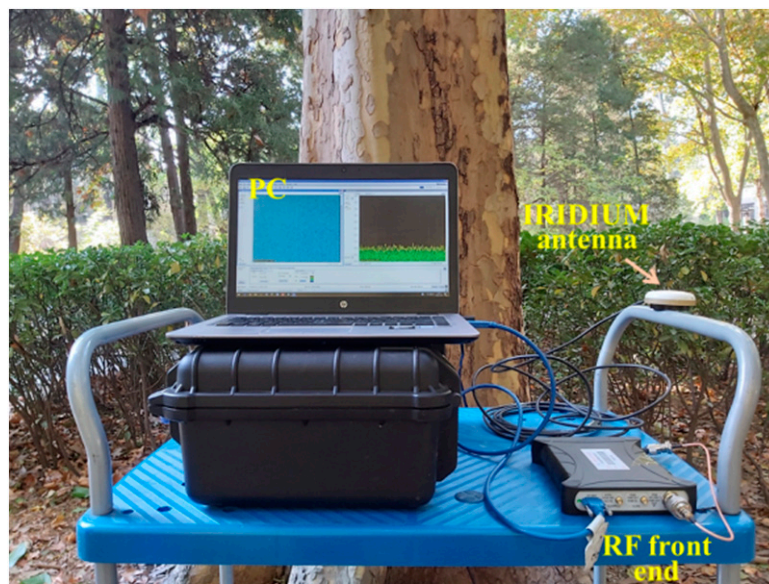
Figure 4. IRIDIUM NEXT data collection in weak signal environment.
