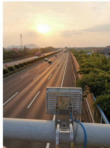
Figure 6. The experimental scene and the placement of the radar.
