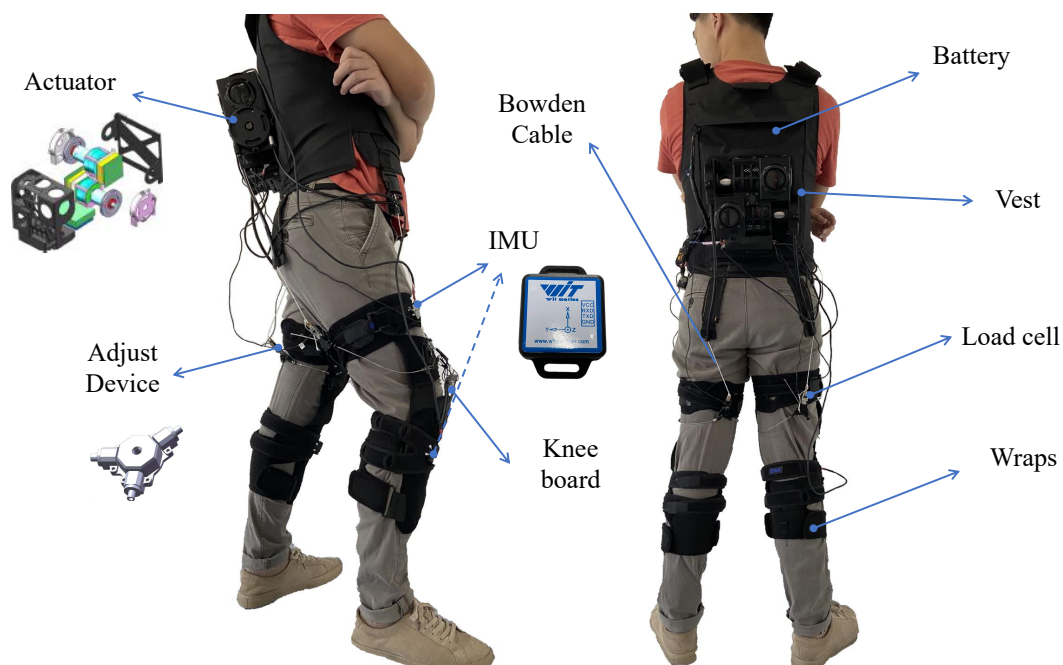
Figure 1. The system overview is showing the structure of the soft exoskeleton and the position of its every part.
