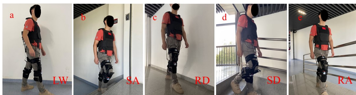
Figure 8. The testers wear a flexible lower-limb exoskeleton to test the continuous terrain motion recognition. (a) LW (Level ground walking), (b) SA (Stair ascent), (c) SD (Stair descent), (d) RA (Ramp ascent), (e) RD (Ramp descent).
