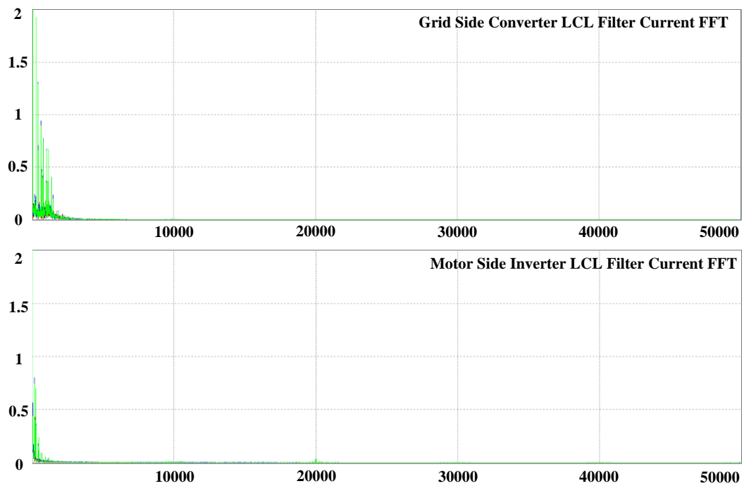
Figure 17. Fast Fourier transform (FFT) analysis results of grid side LCL filter current and motor side current using the conventional SVPWM with the dead time.
