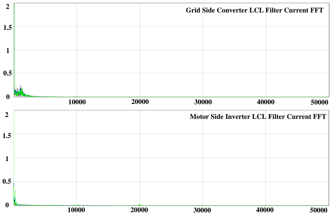
Figure 20. FFT analysis results of grid side LCL filter current and motor side current using the proposed ZDPWM method.
