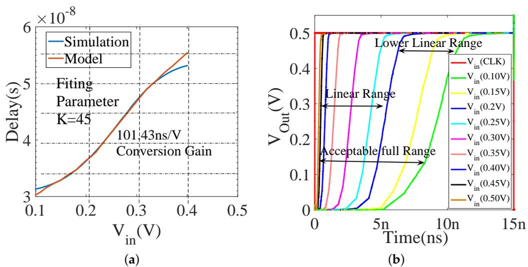
Figure 5. (a) V-T conversion characteristics (b) Output vs. time curve.
