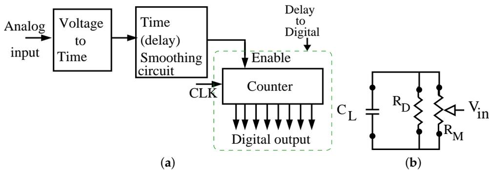
Figure 2. (a) Proposed voltage to time converter (VTC)-based ADC (b) Fundamental Model.
