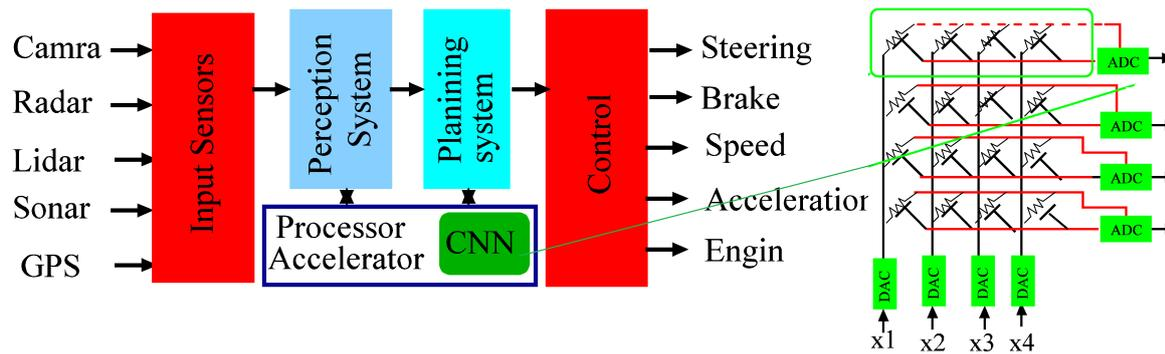
**Figure 1.** Vehicle automation system and use of convolution network-based accelerator using analog to digital converter (ADC).
