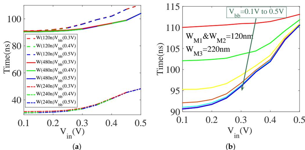
**Figure 7.** Optimization of (a) the transistor widths of controlling circuit and (b) biasing voltage ( $V_{bb}$ ).
