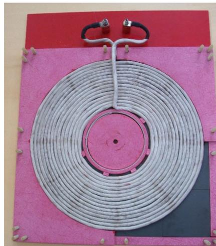
**Figure 9.** Coil without protective cover.
