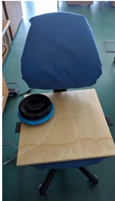
Figure 4. Load cells calibration setup performed using a graduate reference surface positioned on the chair LP and known loads.
