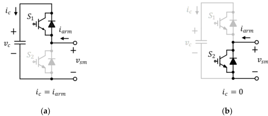
Figure 9. Capacitor current flow diagram. (a) When the SM is inserted; (b) When the SM is bypassed.
