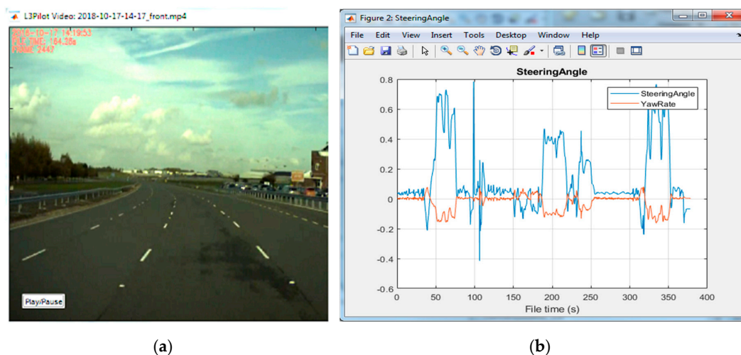
Figure 5. Snapshots from the viewer tool for video data annotation, showing (a) the front camera video, and (b) the steering angle and yaw rate signals in the scene.
