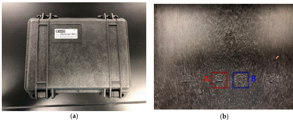
Figure 4. Visual photograph of (a) the polypropylene composite Pelican case and (b) the bumped markings, A and B.
