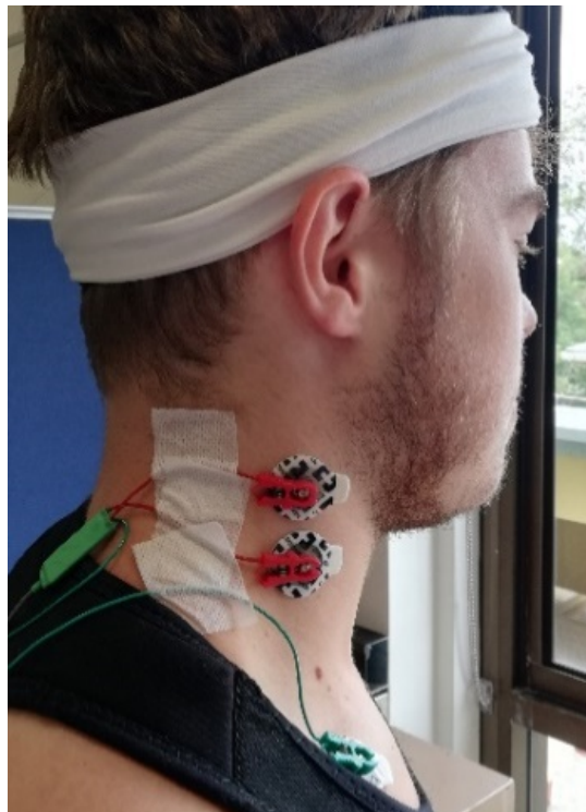
Figure 3. A bipolar electrode configuration over the sternocleidomastoid muscle and a reference electrode placed over the clavicle. A sports bra and headband fixed the position of the inertial sensors.
