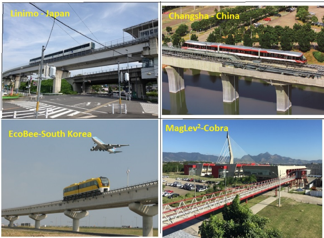
Figure 5. Comparison of MagLev Electromagnetic Levitation (EML) in urban commercial operation in Japan, China, South Korea with the MagLev 2 -Cobra experimental line, which uses SML levitation: lighter and slender.
