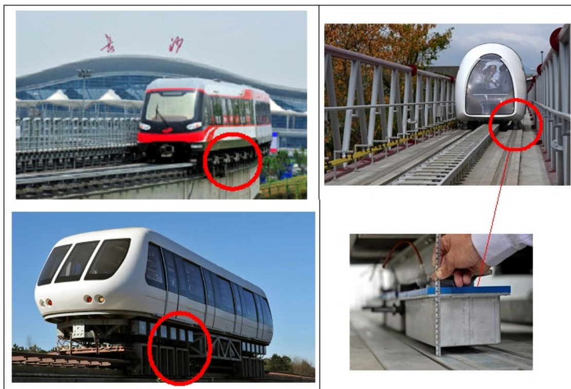
Figure 6. Comparison of the system required to obtain EML levitation (left side) with the cryostats required for MagLev 2 -Cobra, which employs SML technology (right side): simpler and more robust.
