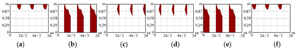
**Figure 4.** The application areas for different modes while  $\varphi = \pi/6$ : (a) Mode 1, (b) Mode 2-1, (c) Mode 2-2, (d) Mode 3-1, (e) Mode 3-2, and (f) Mode 4.
