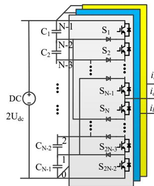
Figure 1. The topology of the diode-clamped multilevel inverter (DCMLI).
