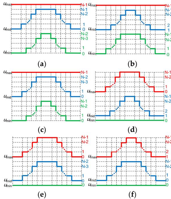
**Figure 2.** The PWM sequences for the FRCVBPWM under different modes: (a) Mode 1, (b) Mode 2-1, (c) Mode 2-2, (d) Mode 3-1, (e) Mode 3-2, and (f) Mode 4.
