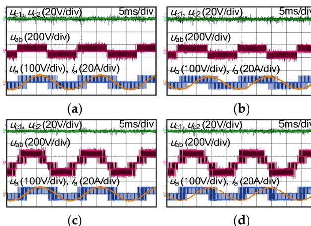
**Figure 10.** Steady state experimental results of virtual space vector pulse width modulation (VSPWM): (a)  $m = 0.3, \varphi = \pi/12$ , (b)  $m = 0.3, \varphi = 5\pi/12$  (c)  $m = 0.9, \varphi = \pi/12$  and (d)  $m = 0.9, \varphi = 5\pi/12$ .
