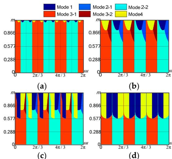
**Figure 7.** The selected modes based on minimum switching loss under several certain values of  $\varphi$ : (a)  $\varphi = 0$ , (b)  $\varphi = \pi/6$ , (c)  $\varphi = \pi/3$ , and (d)  $\varphi = \pi/2$ .
