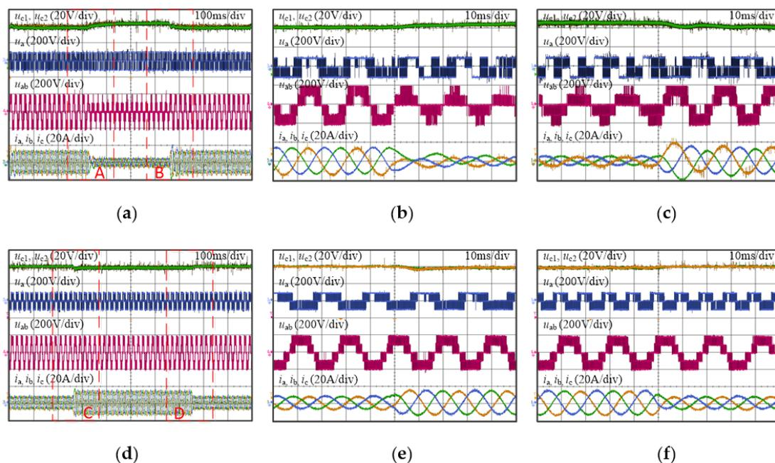
**Figure 14.** Dynamic experimental results of FRCVBPWM: (a) a sudden change of  $m$  between 0.7 and 0.9, (b) partially enlarged waveforms of region A, (c) partially enlarged waveforms of region B, (d) a sudden change of load, (e) partially enlarged waveforms of region C, and (f) partially enlarged waveforms of region D.
