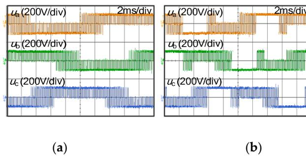
**Figure 13.** The waveforms of three phases voltage for FRCVBPWM and VSVPWM: (a) VSVPWM, and (b) FRCVBPWM.
