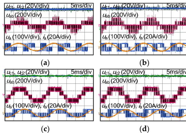
**Figure 11.** Steady state experimental results of FRCVBPWM: (a)  $m = 0.3, \varphi = \pi/12$ , (b)  $m = 0.3, \varphi = 5\pi/12$ , (c)  $m = 0.9, \varphi = \pi/12$ , and (d)  $m = 0.9, \varphi = 5\pi/12$ .
