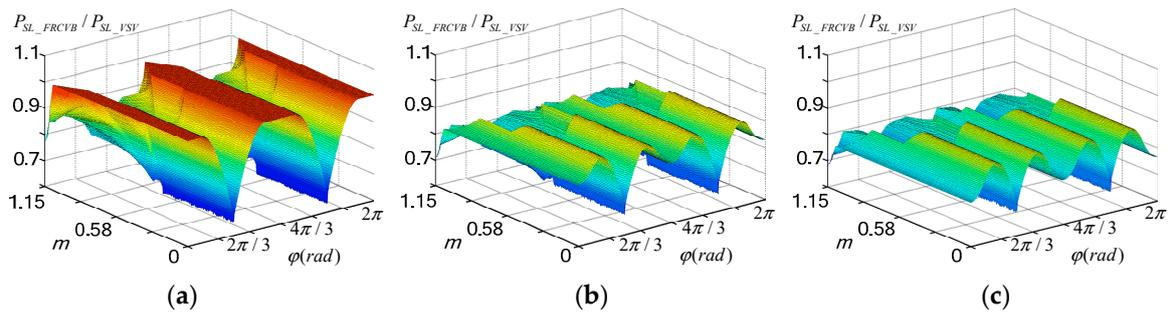
**Figure 9.** The duty ratios of  $P_{SL\_FRCVB}$  to  $P_{SL\_VSV}$  under different levels: (a) three-level, (b) four-level, and (c) five-level.
