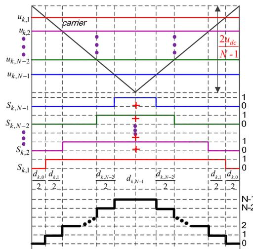
Figure 8. Realization of FRCVBPWM based on the carrier-based PWM.
