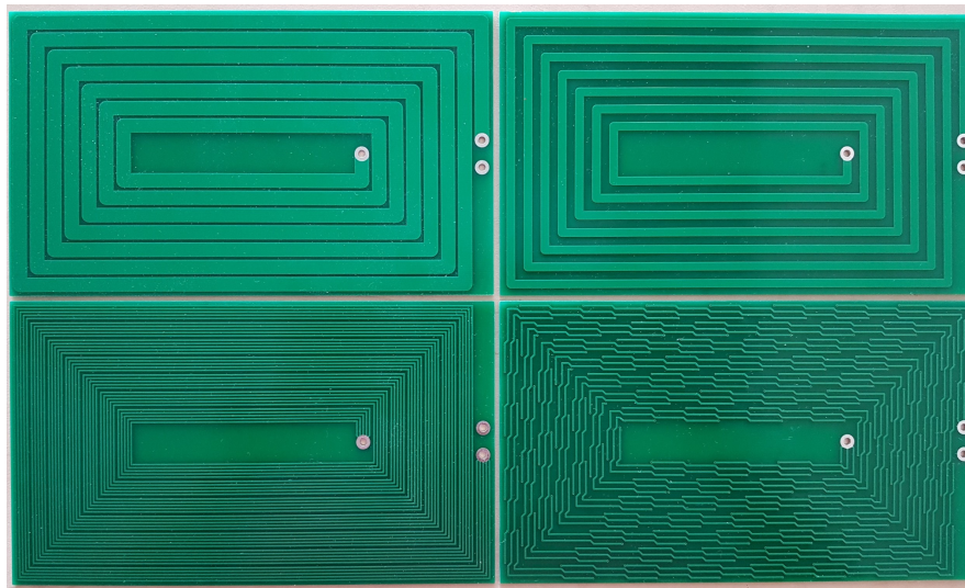
Figure 15. Seven-turn PCB windings with solid 5 mm (Top left), solid 3 mm (Top right), multi-strands (bottom left) and Litz style (bottom right).
