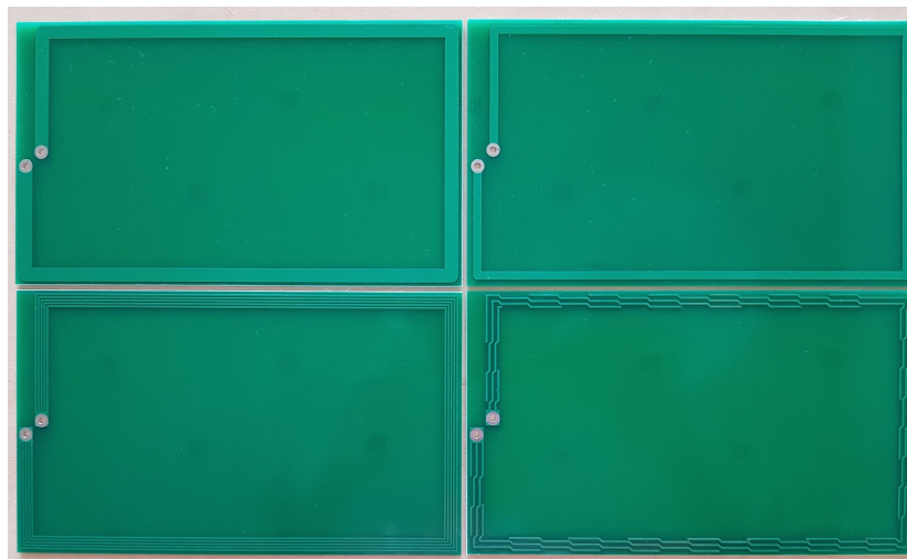
Figure 7. Single turn PCB windings with solid 5 mm (Top Left), solid 3 mm (Top Right), multi-strands (Bottom Left) and Litz style (Bottom Right).
