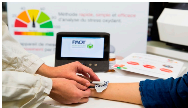
Figure 1. Photography of the electrochemical equipment (Oxystress Analyzer) allowing the measurement of SOSS in a non-invasive way. For details, see the Material and Methods section.
