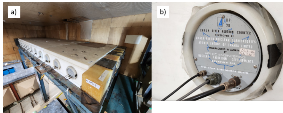
Figure 7. Photograph of the neutron monitor located at Mt. Norikura cosmic ray observatory (2778 m) (a) and the \text{BF}_3 counter (Chalk River neutron counter) (b).
