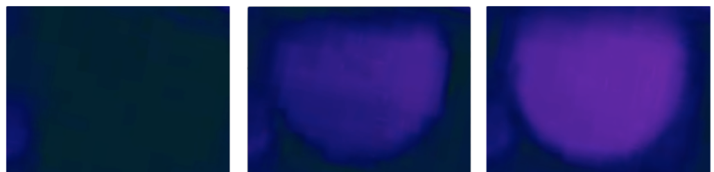
Figure 5. Thermal imaging capture of supercooled WbLS freezing. These three example frames are ordered chronologically from left to right and are taken from a 25-second-long clip. The color black is approximately -19 °C, while the purple coloration is 0 ° on the FLIR unit's internally calibrated, automatically adjusting scale. The purple-colored artifact present in all images on the left is ice build-up on a thermocouple cable, in the open-air chiller used at BNL. One can see the hemispherical bottom of the test tube come into view very slowly, whereas it was entirely invisible (black) at the start, in thermal equilibrium with the cold air surrounding the vessel. (Note that the top oil was already frozen).
