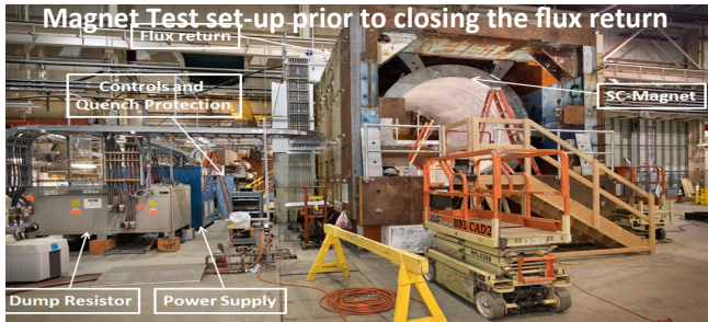
Figure 9. BABAR superconducting solenoid now in operation at BNL.
