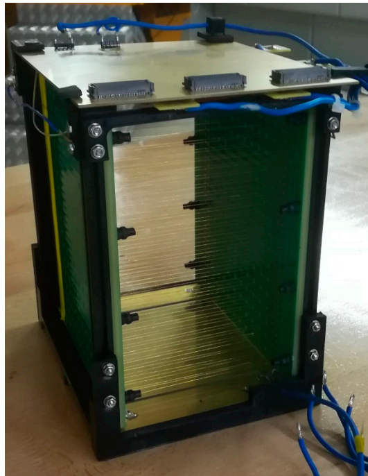
Figure 9. One of the eight modules of the gas tracker, which has been used as prototype for testing purposes.
