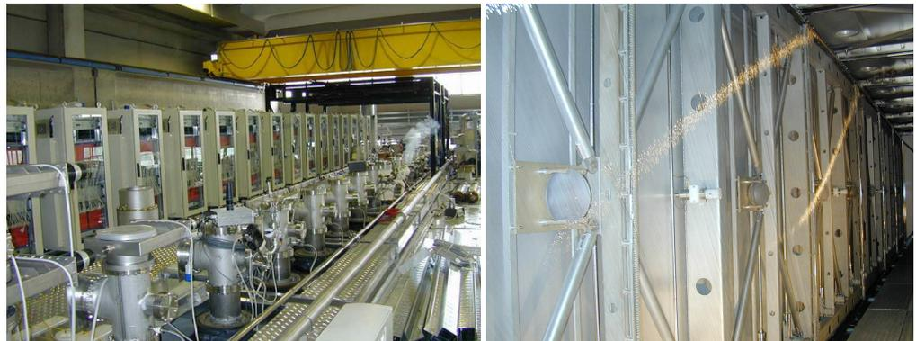
**Figure 6.** (Left): Top of one module of ICARUS-T600 in the Pavia surface laboratory, showing the disposition of the electronic racks for the one TPC and of the chimneys with the feed-through flanges for the other TPC. (Right): Inner detector of one module of ICARUS-T600, showing the wire chamber structure and the PMTs behind.
