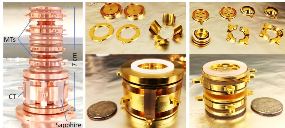
Figure 6. Pictures of the CHIP-TRAP Penning traps. Left: the assembled hyperbolic measurement traps stacked on top of the capture trap before the electrodes were gold plated. Middle: the cylindrical capture trap after gold plating, consisting of two end caps, two correction ring electrodes and quartered ring electrodes. Right: the hyperbolic measurement traps after gold plating, consisting of hyperbolic ring and end-cap electrodes, quartered correction ring electrode and correction tube electrodes. The two traps are stacked together in the bottom picture. Sapphire insulating rings can also be seen in the pictures.
