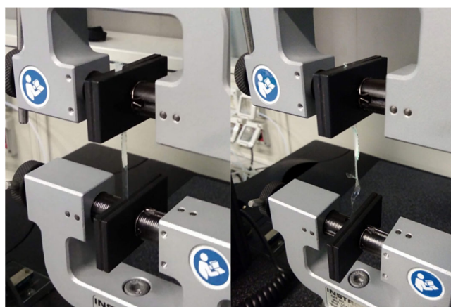
Figure S5. Pictures of Keratin/PBS50/50 (left) and PBS (right) electrospun mats during shear strength measurements.
