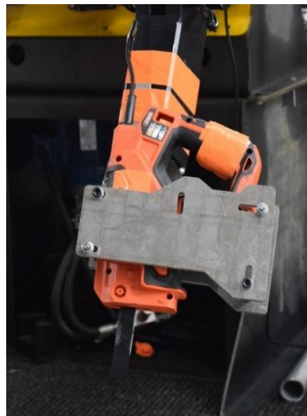
Figure 4. The reciprocating saw mounted on the arm equipped with metal cutting blade.
