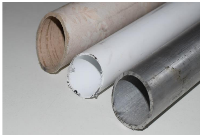
Figure 7. The cut surface of the three pipes (left to right): cardboard, plastic and aluminium.
