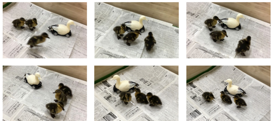
Figure 5. Follow behavior displayed after imprinting. Baby mallards followed the robot that moved slowly.
